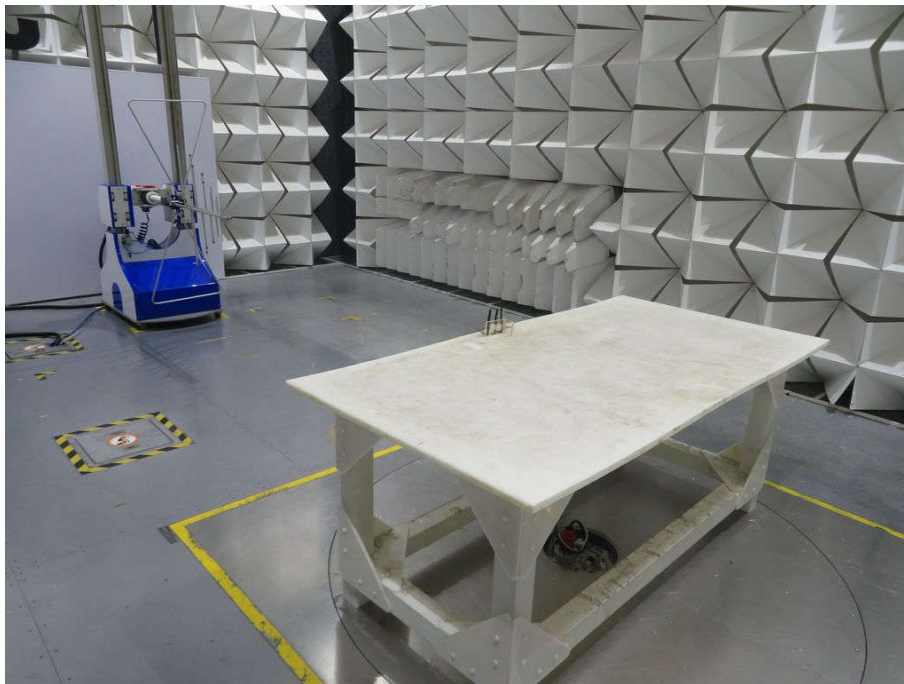
Radiated emission Test Setup-1(Below 1GHz)
