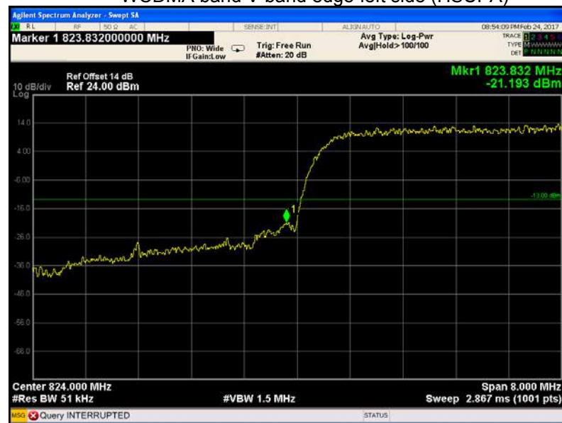
WCDMA band V band edge-left side (HSUPA)
