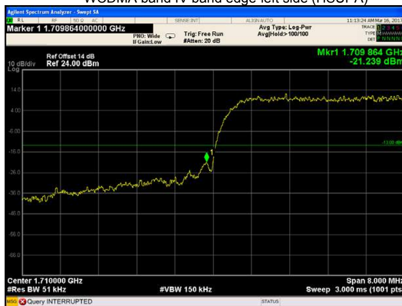
WCDMA band IV band edge-left side (HSUPA)
