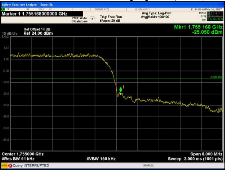
WCDMA band IV band edge-right side (HSUPA)
