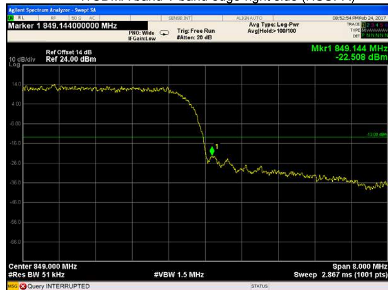
WCDMA band V band edge-right side (HSUPA)
