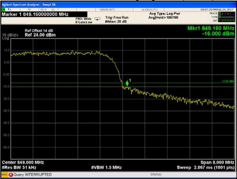
WCDMA band V band edge-right side (HSUPA)
