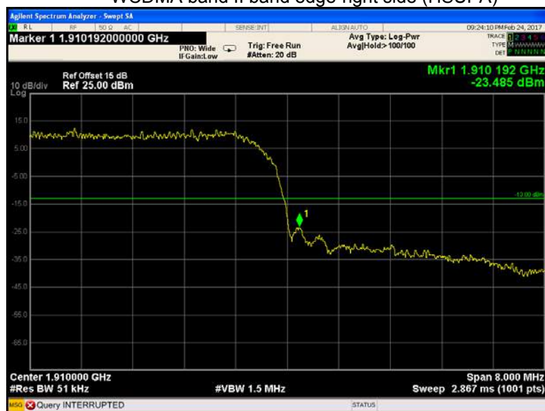
WCDMA band II band edge-right side (HSUPA)
