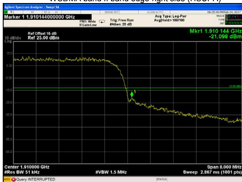
WCDMA band II band edge-right side (HSUPA)
