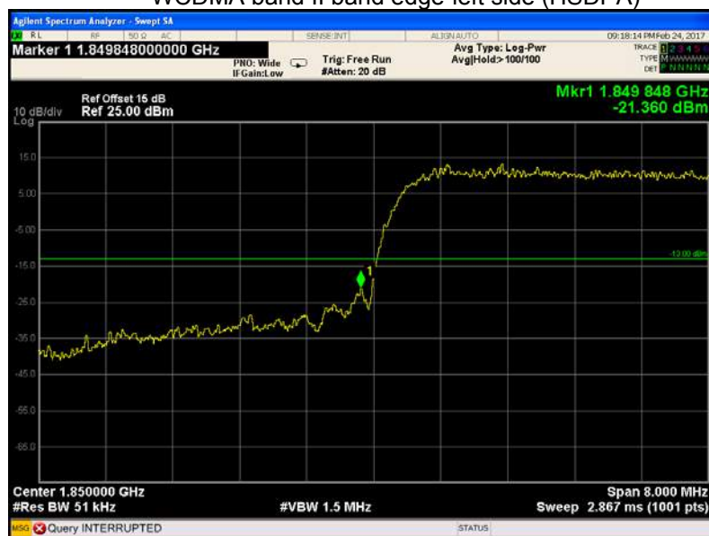
WCDMA band II band edge-left side (HSDPA)
