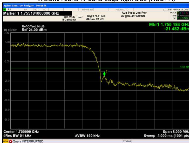
WCDMA band IV band edge-right side (HSUPA)
