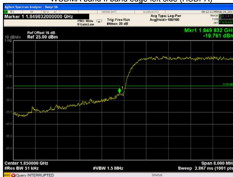
WCDMA band II band edge-left side (HSDPA)
