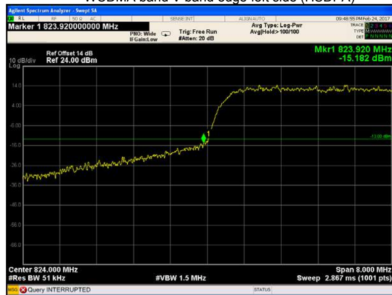
WCDMA band V band edge-left side (HSDPA)
