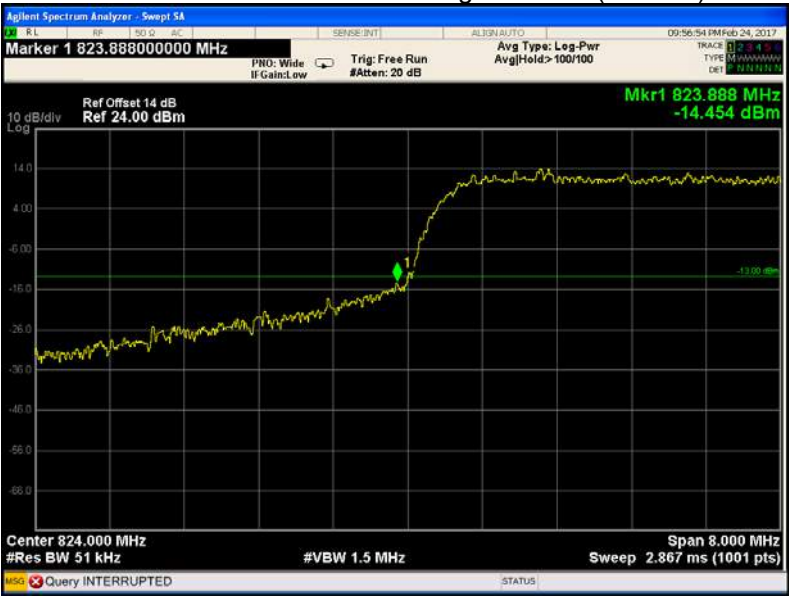
WCDMA band V band edge-left side (HSUPA)
