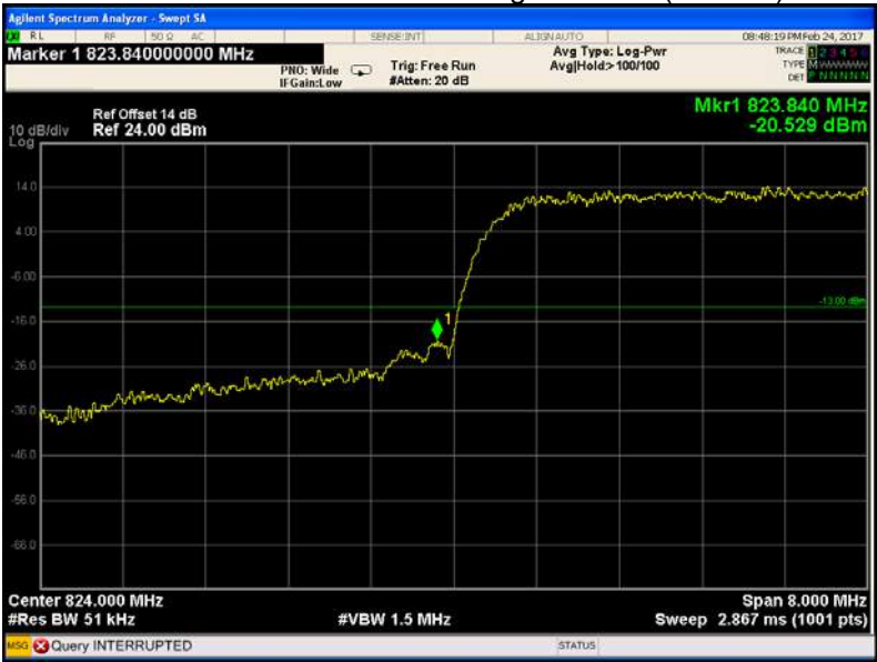
WCDMA band V band edge-left side (HSDPA)
