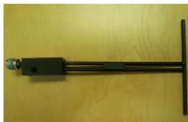
Figure 1 – MVG COMOSAR Validation Dipole
