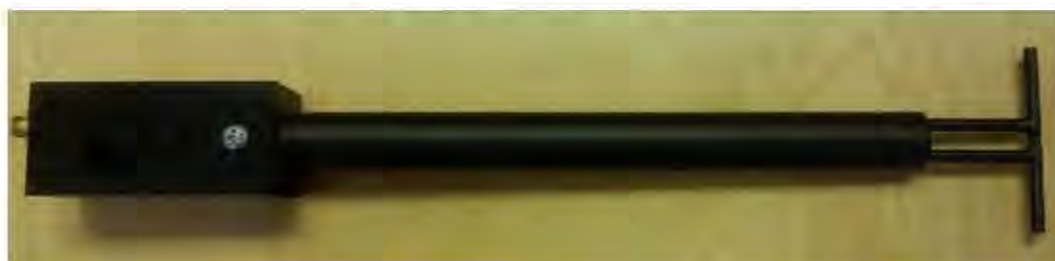
Figure 1 – MVG COMOSAR Validation Dipole
