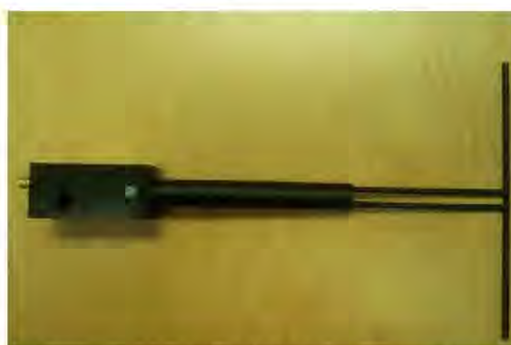
Figure 1 – MVG COMOSAR Validation Dipole
