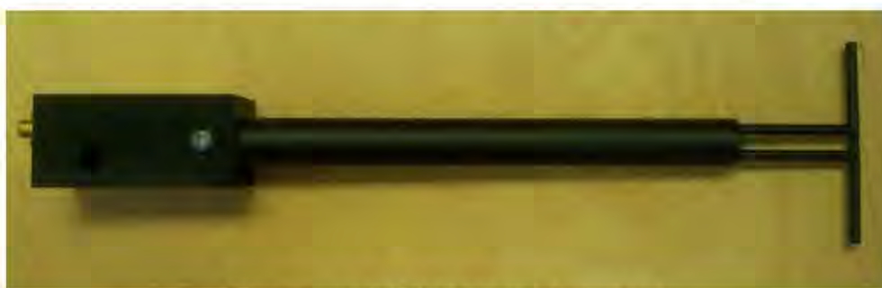
Figure 1 – MVG COMOSAR Validation Dipole
