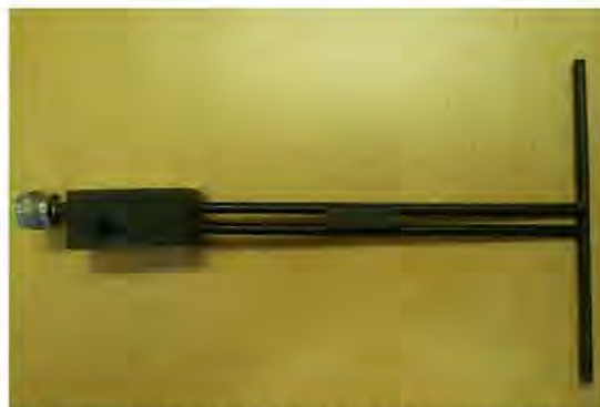
Figure 1 – MVG COMOSAR Validation Dipole
