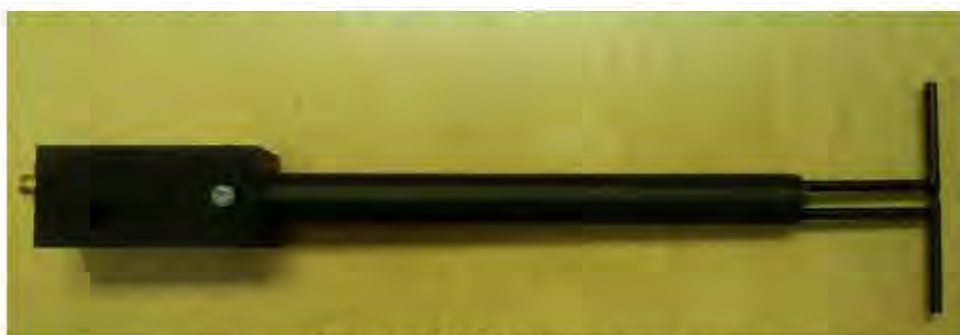
Figure 1 – MVG COMOSAR Validation Dipole
