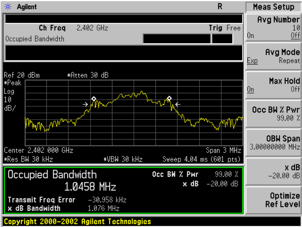
TEST PLOT OF BANDWIDTH FOR LOW CHANNEL
