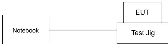
This example is connection diagram of EUT test configurations.
