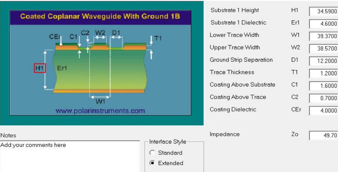
Figure 2: Grand referring to layer 4 Finished Copper, 39.37 mil
