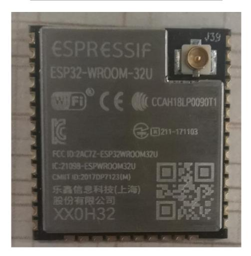
The device is unique 'antenna connector, and type is IPEX.
