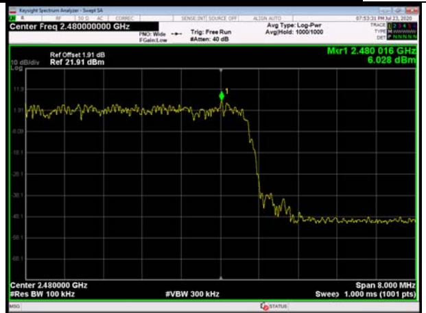
BT 3DH5 CH78, Carrier frequency (MHz): 2480
