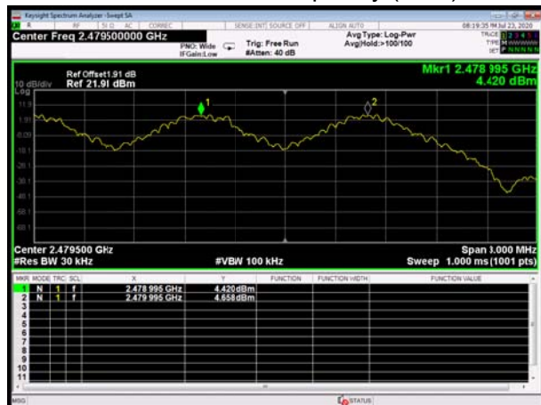
BT DH5 CH78, Carrier frequency (MHz): 2480
