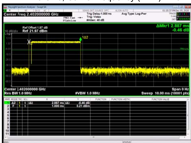
BT 2DH5 CH39, Carrier frequency (MHz): 2441
