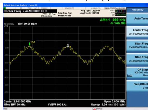
BT DH5 CH78, Carrier frequency (MHz): 2480
