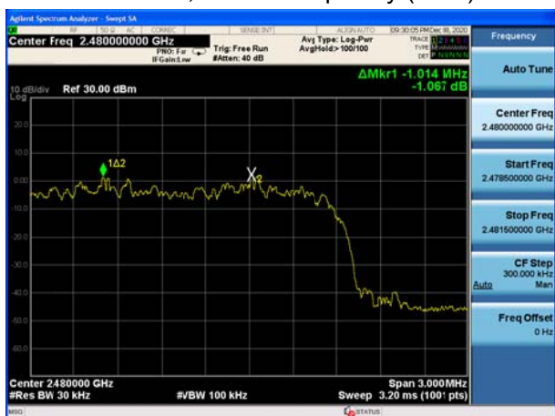
BT 2DH5 CH78, Carrier frequency (MHz): 2480
