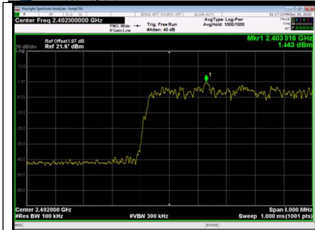
BT 3DH5 CH0, Carrier frequency (MHz): 2402
