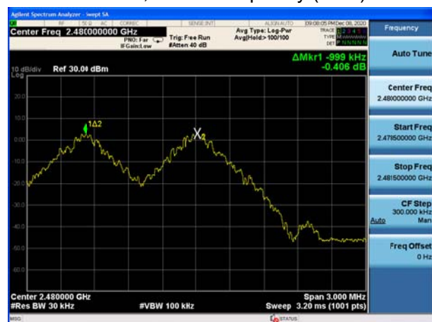
BT DH5 CH78, Carrier frequency (MHz): 2480
