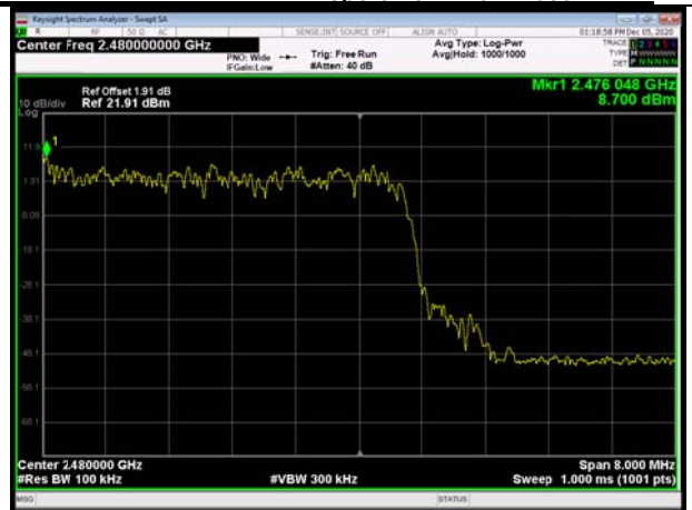
BT 3DH5 CH78, Carrier frequency (MHz): 2480
