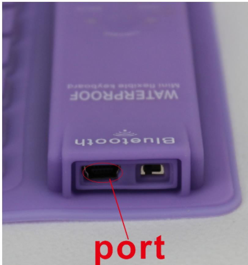
2. Firstly, take out the USB charging cable from the purchase attachment, plug the male side into the computer's USB port, and plug the other side into the keyboard's charging port, when charging the charging indicator will showed with red color, as below:
