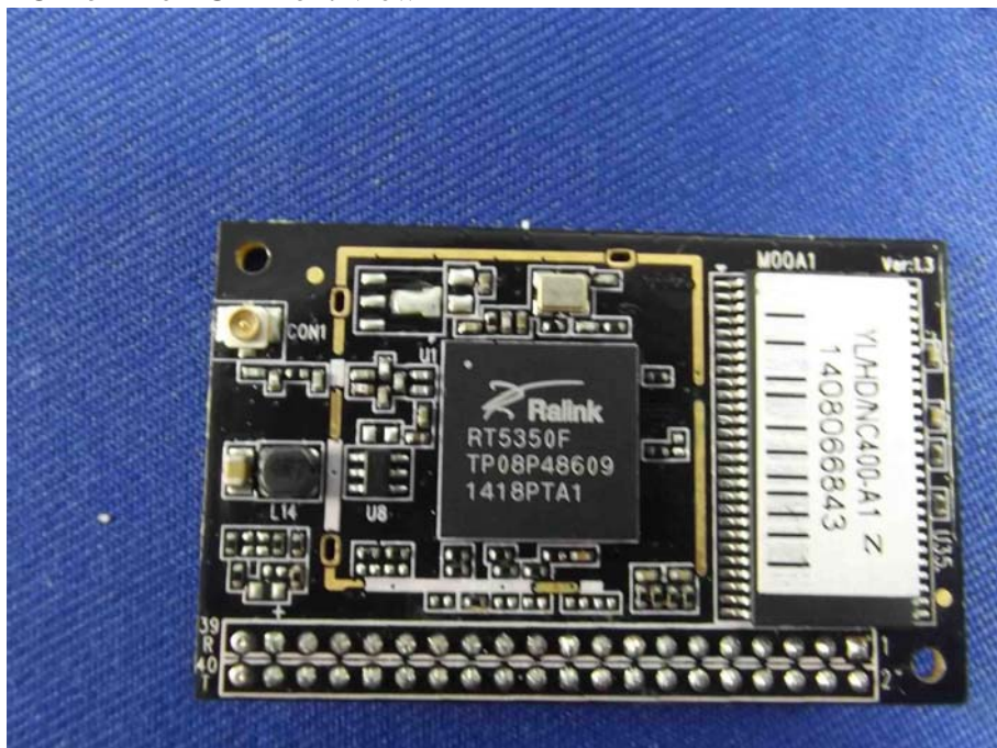
Figure 12 PCB of The EUT-Front View
