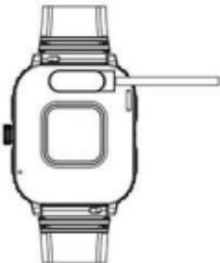
Connect and charge the watch according to the picture. It needs to be charged to activate the watch when it is started for the first time.
