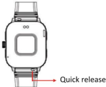
Remove the strap from the watch by sliding the quick release on the strap.
