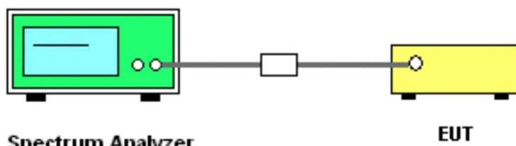
Picture 17: Test setup for occupied bandwidth measurement
