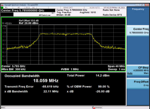
U-NII-3 99% Bandwidth-802.11ac(20MHz) ,5785MHz,Ant1
