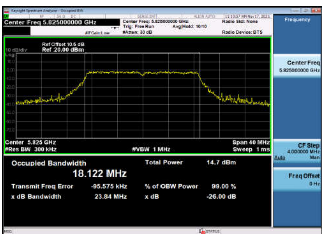
U-NII-3 99% Bandwidth-802.11n(20MHz) ,5825MHz,Ant1
