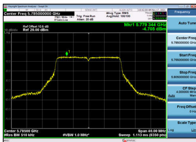
U-NII-3 Power spectral density-802.11 a(20MHz),5785MHz,Ant1
