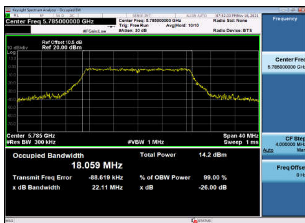
U-NII-3 99% Bandwidth-802.11ac(20MHz) ,5785MHz,Ant1
