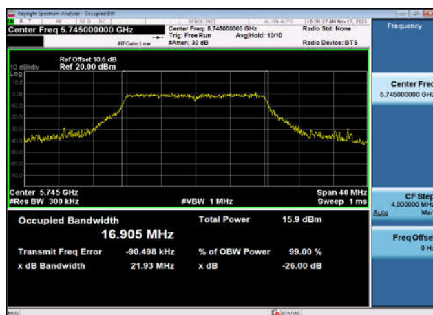
U-NII-3 99% Bandwidth-802.11a(20MHz) ,5825MHz,Ant1
