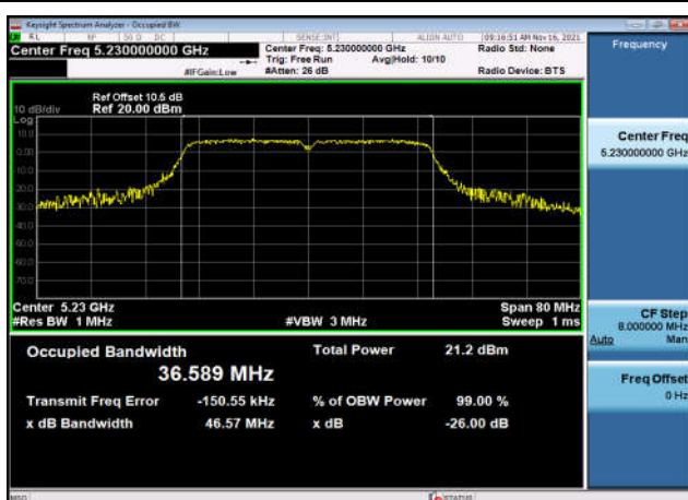
U-NII-1 99% Bandwidth-802.11n(40MHz) ,5230MHz,Ant1
