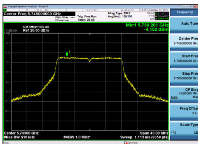
U-NII-3 Power spectral density-802.11 a(20MHz),5825MHz,Ant1
