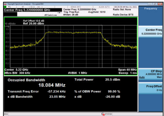
U-NII-1 99% Bandwidth-802.11n(40MHz) ,5190MHz,Ant1
