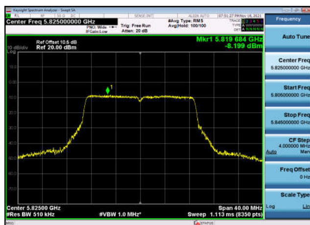
U-NII-3 Power spectral density-802.11 ac(40MHz),5795MHz,Ant1
