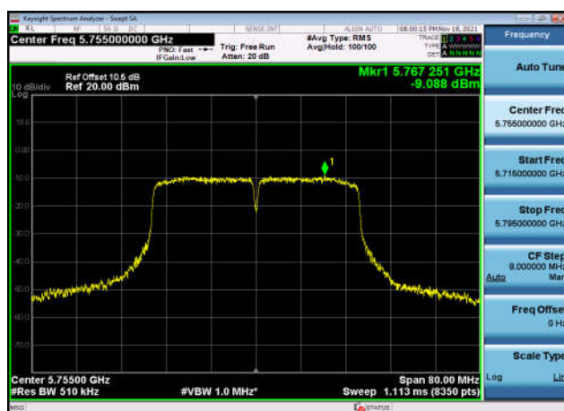
U-NII-3 Power spectral density-802.11 ac(80MHz),5775MHz,Ant1
