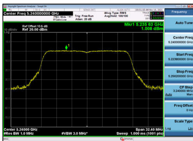
U-NII-1 Power spectral density-802.11 ac(20MHz),5240MHz,Ant1
