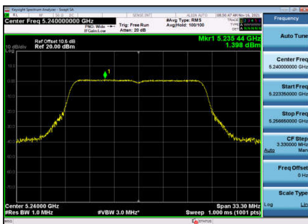
U-NII-1 Power spectral density-802.11 n(40MHz),5230MHz,Ant1
