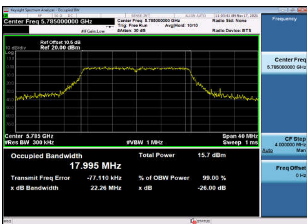
U-NII-3 99% Bandwidth-802.11n(40MHz) ,5755MHz,Ant1
