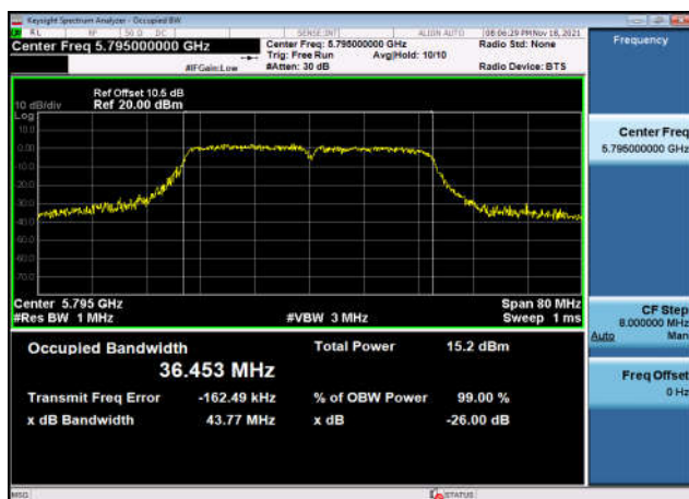
U-NII-3 99% Bandwidth-802.11ac(40MHz) ,5795MHz,Ant1
