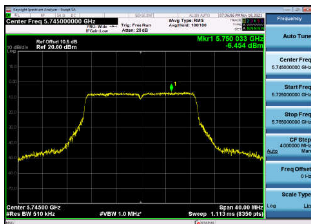
U-NII-3 Power spectral density-802.11 ac(20MHz),5825MHz,Ant1
