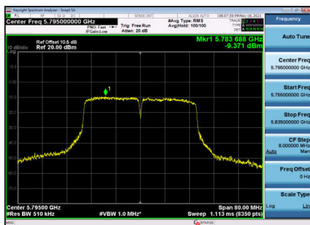
U-NII-3 Power spectral density-802.11 ac(40MHz),5795MHz,Ant1
