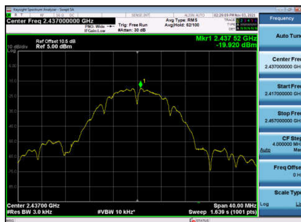
Power spectral density-802.11g ,2412MHz,Ant0
