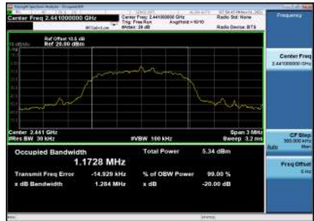
20dB Bandwidth: 8DPSK,2441MHz,3DH5
