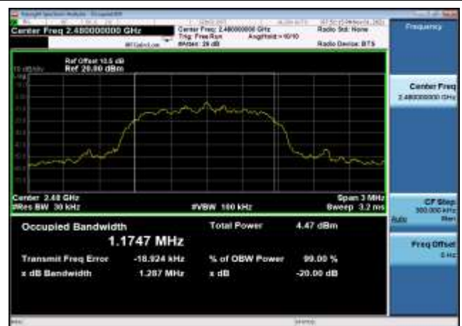
20dB Bandwidth: DQPSK,2480MHz,2DH5
