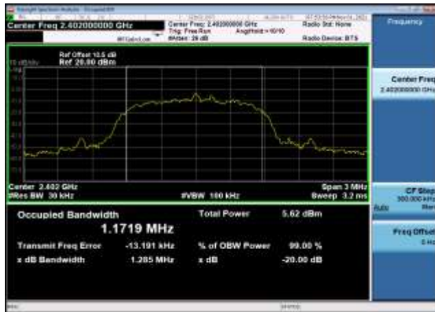
20dB Bandwidth: 8DPSK,2480MHz,3DH5
