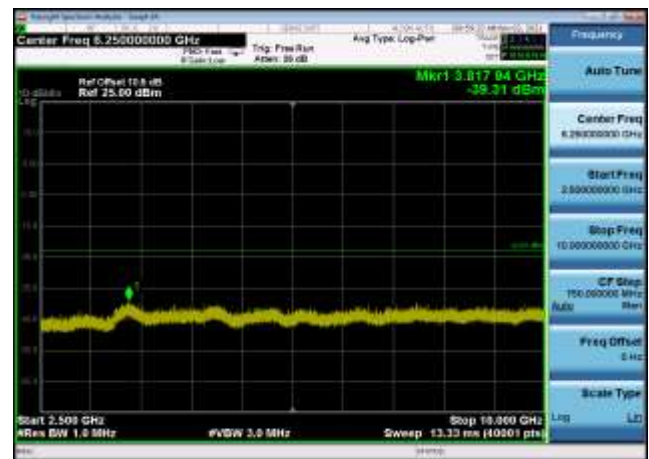
Conducted Emission: 8DPSK,2480,3DH5 ,2500MHz~10000MHz
