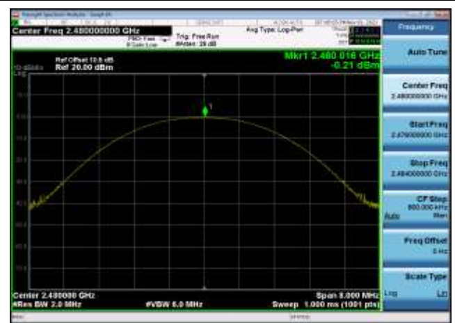
Output Power: DQPSK,2480MHz,2DH5
