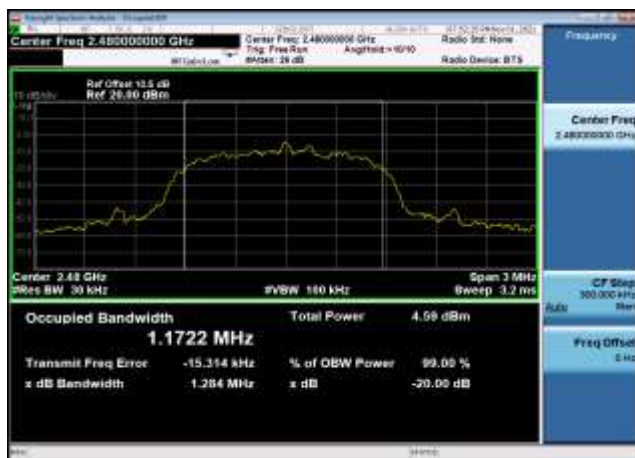
20dB Bandwidth: 8DPSK,2480MHz,3DH5
