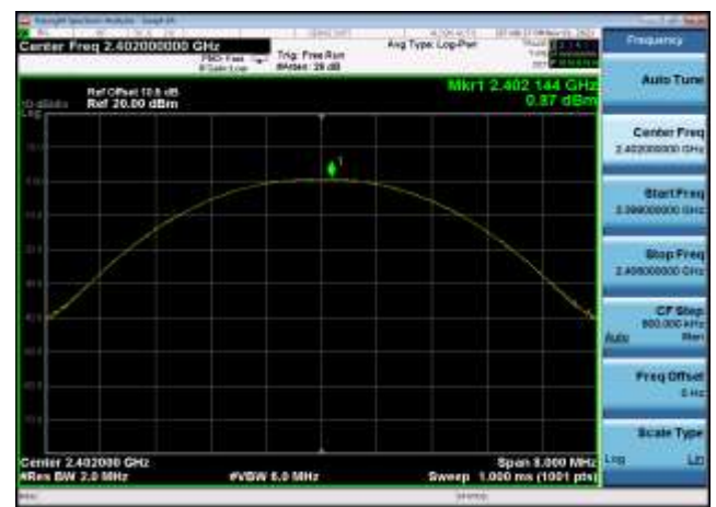
Output Power: DQPSK,2480MHz,2DH5
