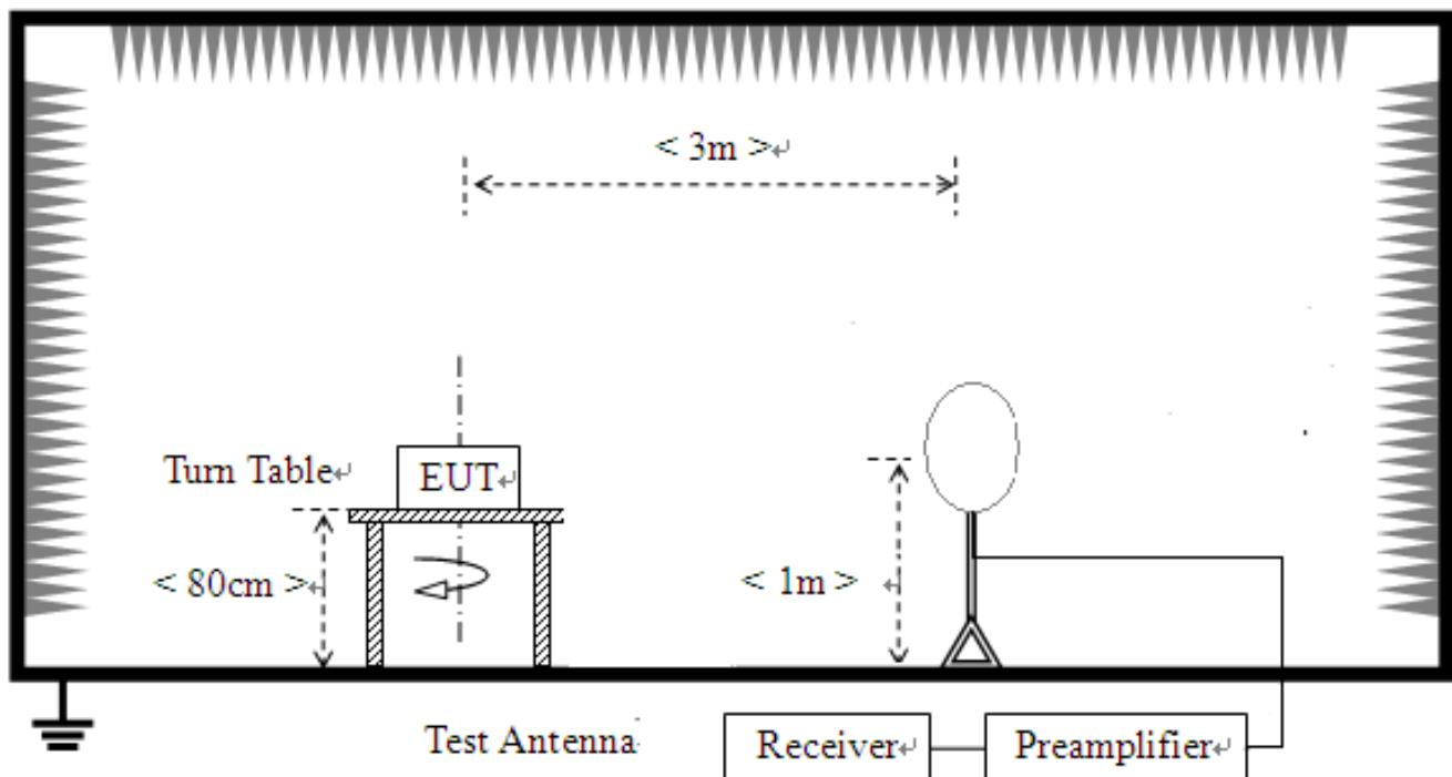
For radiated emissions from 30MHz to 1GHz
