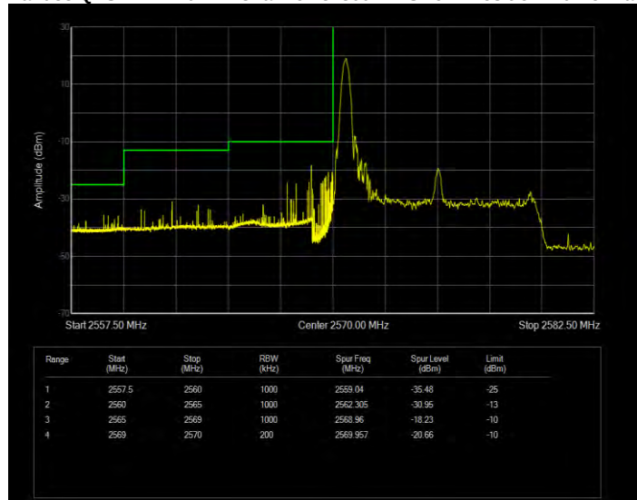
Band38 QPSK BW=10MHz Channel=37800 RB Size=1 Position=#Max Extended
