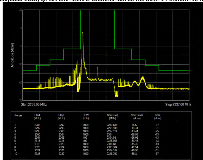
Band40(2305-2315) QPSK BW=10MHz Channel=38750 RB Size=50 Position=#0 Extended
