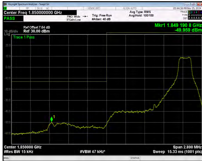
Band2 QPSK BW=1.4MHz Channel=18607 RB Size=6 Position=#0 Extended
