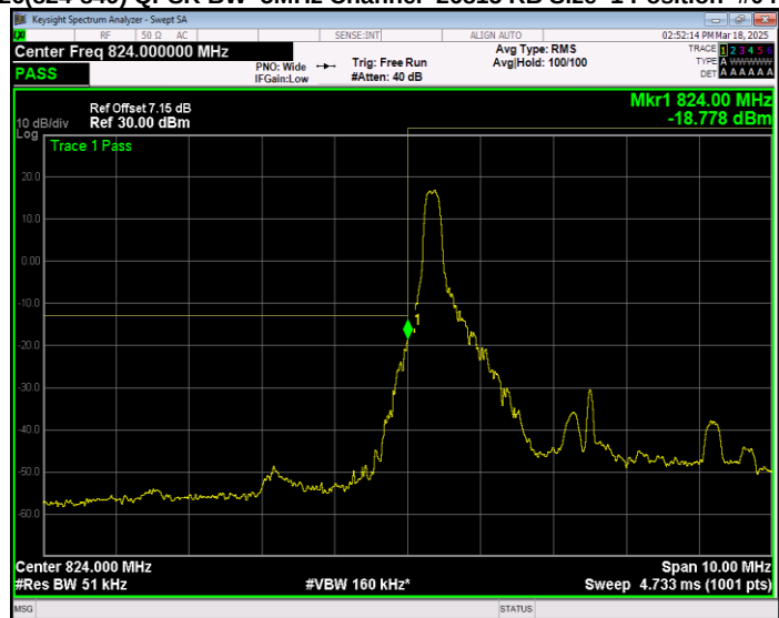
Band26(824-849) QPSK BW=5MHz Channel=26815 RB Size=1 Position=#Max Extended
