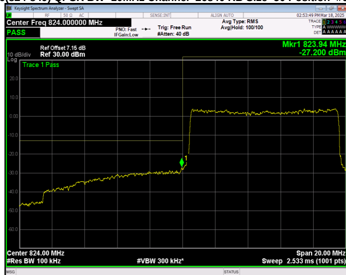
Band26(824-849) QPSK BW=10MHz Channel=26990 RB Size=1 Position=#0 Extended
