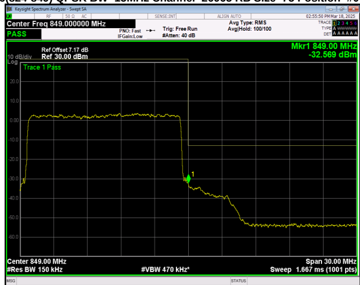
Band26(824-849) QPSK BW=15MHz Channel=26965 RB Size=75 Position=#0 Extended
