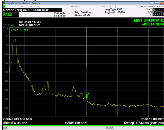
Band26(824-849) 16QAM BW=5MHz Channel=27015 RB Size=1 Position=#Max Extended
