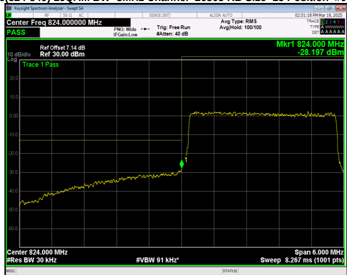
Band26(824-849) 16QAM BW=3MHz Channel=27025 RB Size=1 Position=#0 Extended
