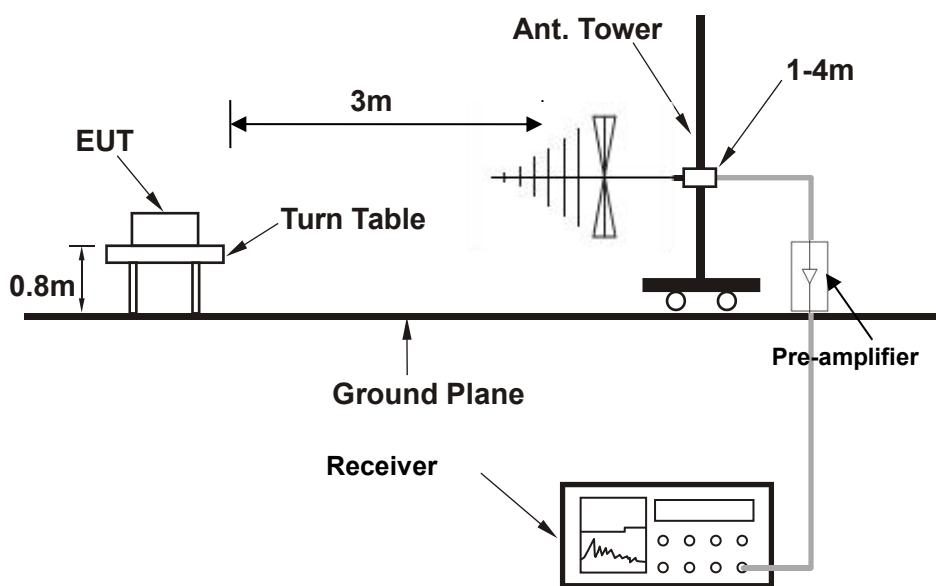
**For radiated test from 1GHz to 18GHz**
