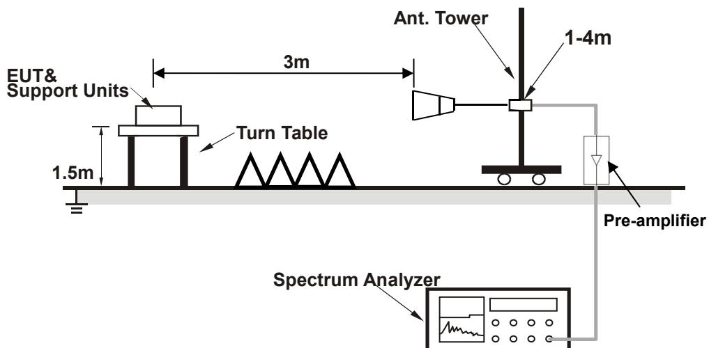
**For radiated test above 18GHz**
