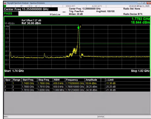
n66 SCS=15kHz DFT_256QAM BW=40MHz HighChannel=352000 RB=1@215
