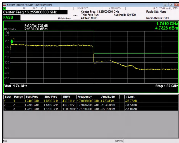
n66 SCS=15kHz DFT_QPSK BW=40MHz HighChannel=352000 RB=216@0
