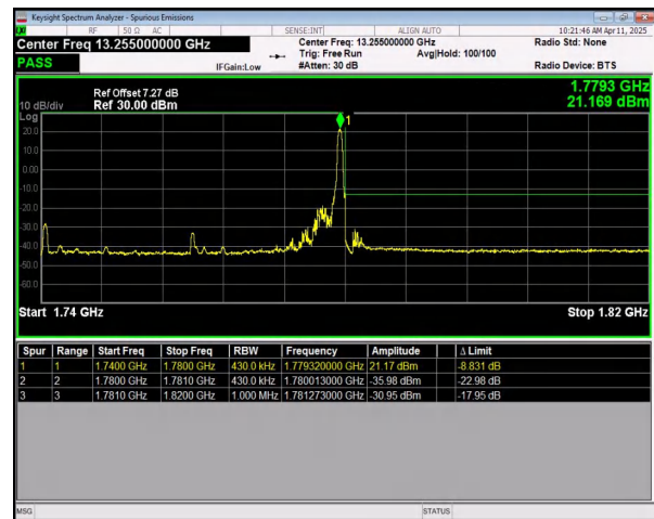
n66 SCS=15kHz DFT_16QAM BW=40MHz HighChannel=352000 RB=1@215
