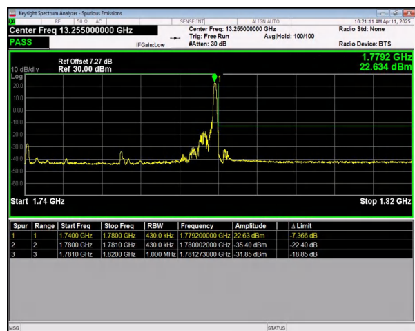
n66 SCS=15kHz DFT_BPSK BW=40MHz HighChannel=352000 RB=1@215
