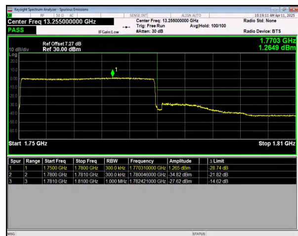
n66 SCS=15kHz CP_QPSK BW=30MHz HighChannel=353000 RB=160@0
