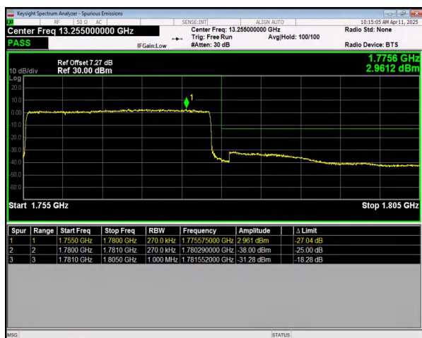
n66 SCS=15kHz DFT_64QAM BW=25MHz HighChannel=353500 RB=128@0
