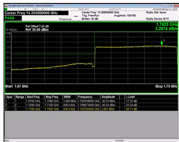
n66 SCS=15kHz DFT_16QAM BW=40MHz LowChannel=346000 RB=216@0
