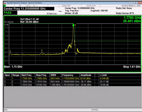
n66 SCS=15kHz DFT_64QAM BW=30MHz HighChannel=353000 RB=1@159
