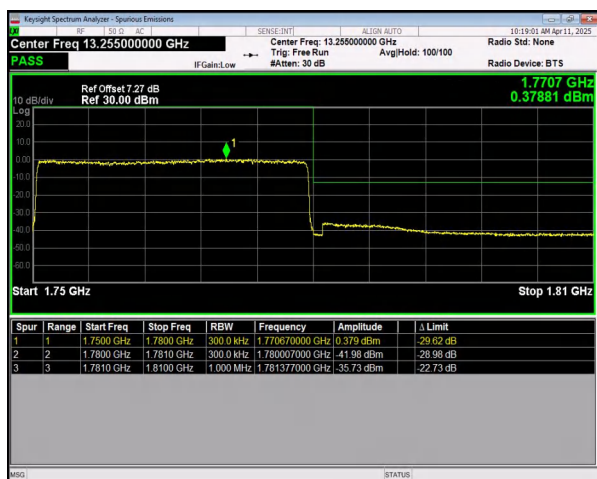
n66 SCS=15kHz DFT_256QAM BW=30MHz HighChannel=353000 RB=160@0
