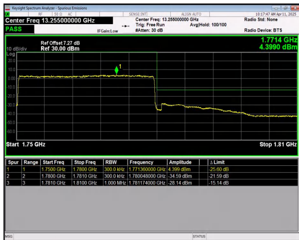
n66 SCS=15kHz DFT_BPSK BW=30MHz HighChannel=353000 RB=160@0
