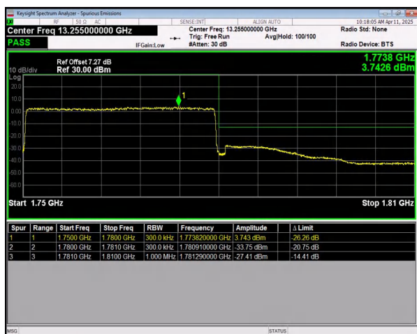
n66 SCS=15kHz DFT_QPSK BW=30MHz HighChannel=353000 RB=160@0
