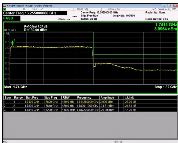
n66 SCS=15kHz DFT_16QAM BW=40MHz HighChannel=352000 RB=216@0
