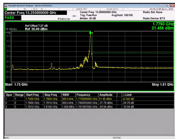
n66 SCS=15kHz DFT_16QAM BW=30MHz HighChannel=353000 RB=1@159
