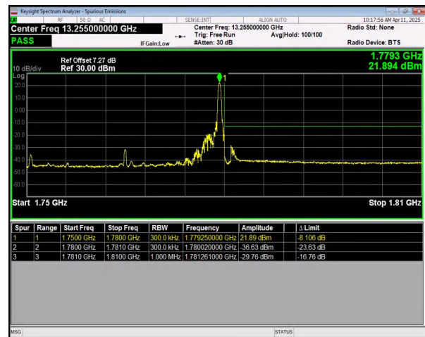
n66 SCS=15kHz DFT_QPSK BW=30MHz HighChannel=353000 RB=1@159
