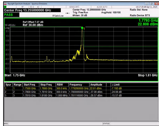
n66 SCS=15kHz DFT_BPSK BW=30MHz HighChannel=353000 RB=1@159
