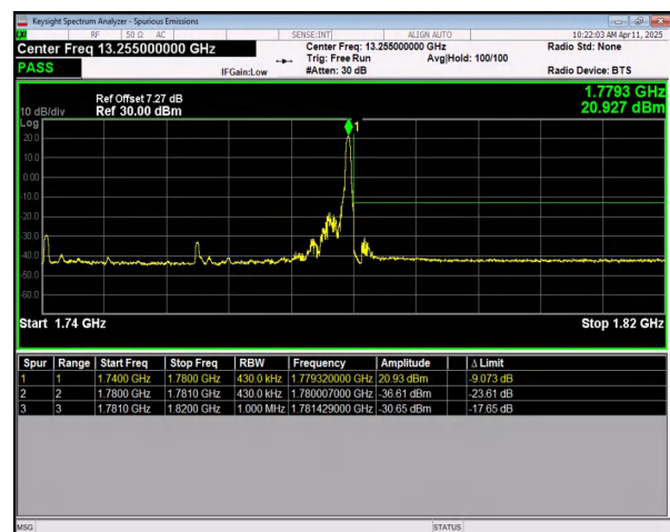
n66 SCS=15kHz DFT_64QAM BW=40MHz HighChannel=352000 RB=1@215
