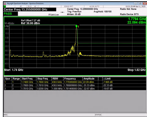
n66 SCS=15kHz DFT_QPSK BW=40MHz HighChannel=352000 RB=1@215
