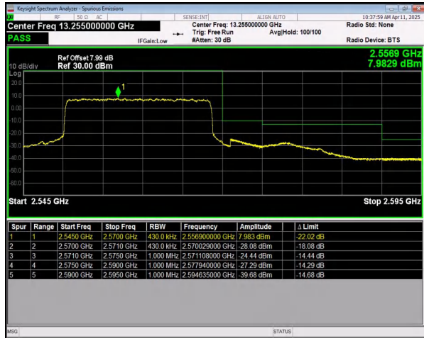
n7 SCS=15kHz DFT_BPSK BW=20MHz HighChannel=512000 RB=100@0
