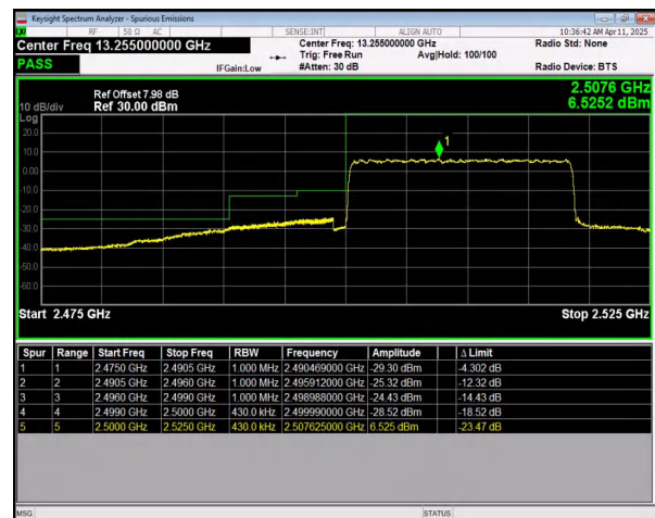
n7 SCS=15kHz DFT_16QAM BW=20MHz LowChannel=502000 RB=100@0
