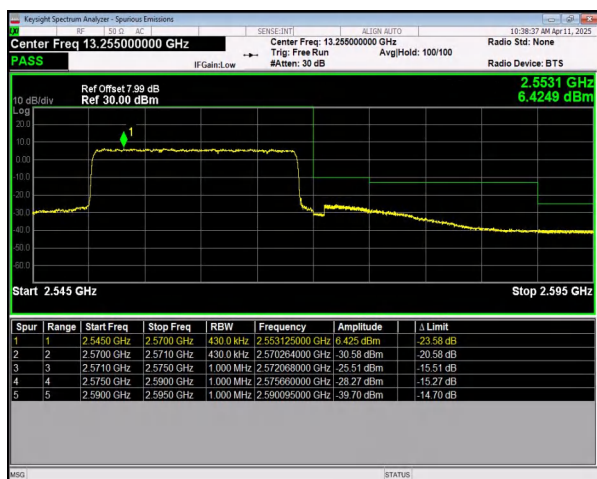
n7 SCS=15kHz DFT_16QAM BW=20MHz HighChannel=512000 RB=100@0
