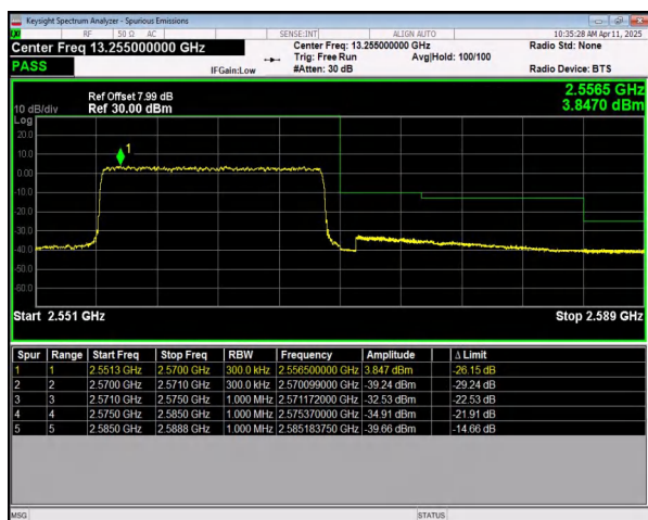
n7 SCS=15kHz DFT_256QAM BW=15MHz HighChannel=512500 RB=75@0
