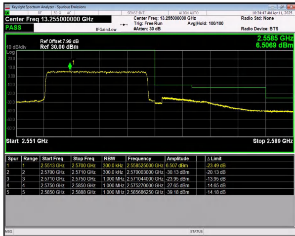
n7 SCS=15kHz DFT_16QAM BW=15MHz HighChannel=512500 RB=75@0
