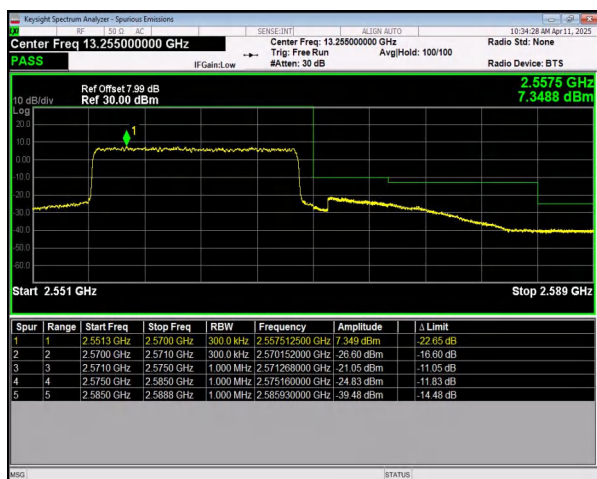
n7 SCS=15kHz DFT_QPSK BW=15MHz HighChannel=512500 RB=75@0
