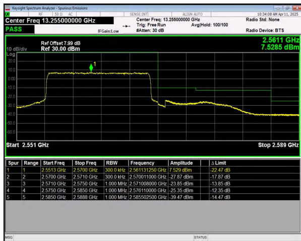
n7 SCS=15kHz DFT_BPSK BW=15MHz HighChannel=512500 RB=75@0
