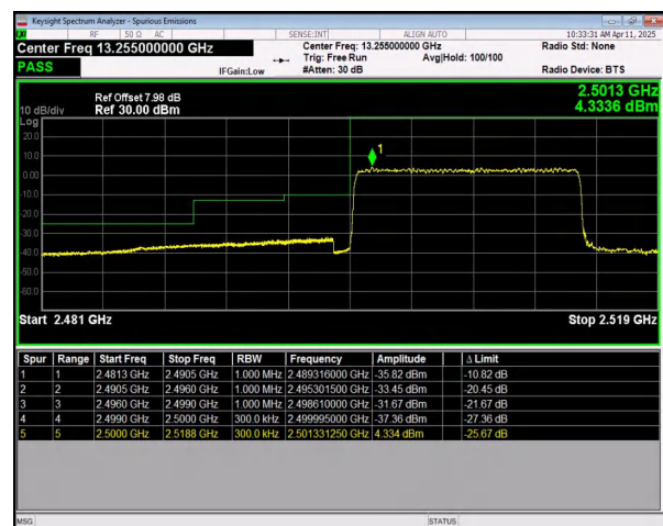
n7 SCS=15kHz DFT_256QAM BW=15MHz LowChannel=501500 RB=75@0
