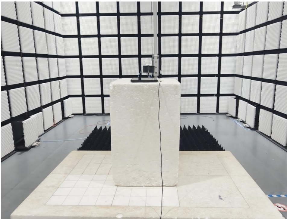
Radiated spurious emission Test Setup-2(Above 1GHz)
