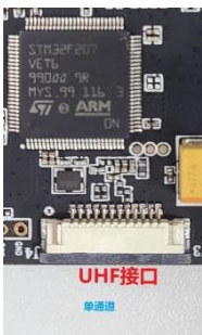
Figure 4.3.2 12-pin single-channel module interface location (Position 5)
