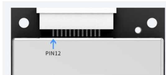
Figure 3.2.1.a Single Channel Module Interface Diagram
