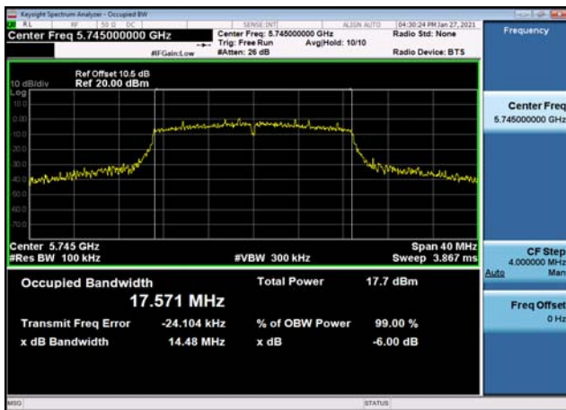
U-NII-3 6dB Bandwidth-802.11n(20MHz) ,5825MHz,Ant1
