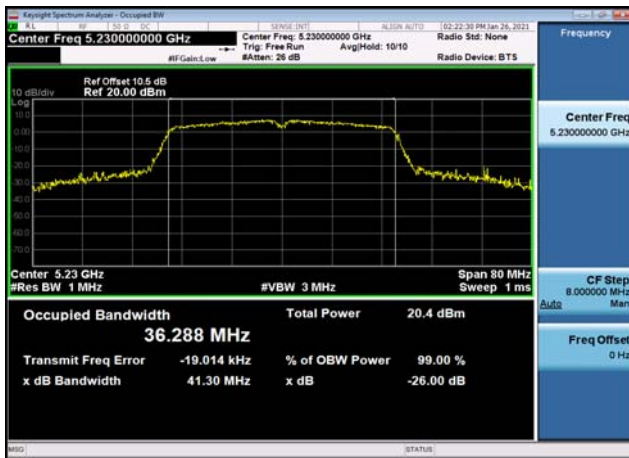
U-NII-2a 99% Bandwidth-802.11n(20MHz) ,5260MHz,Ant1
