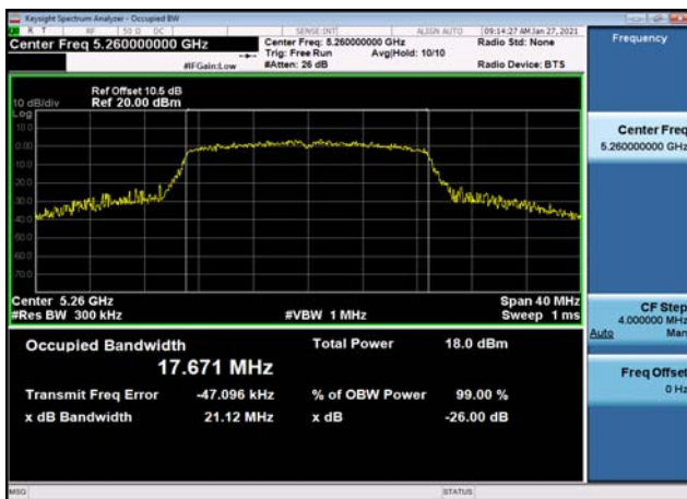
U-NII-2a 99% Bandwidth-802.11n(20MHz) ,5320MHz,Ant1
