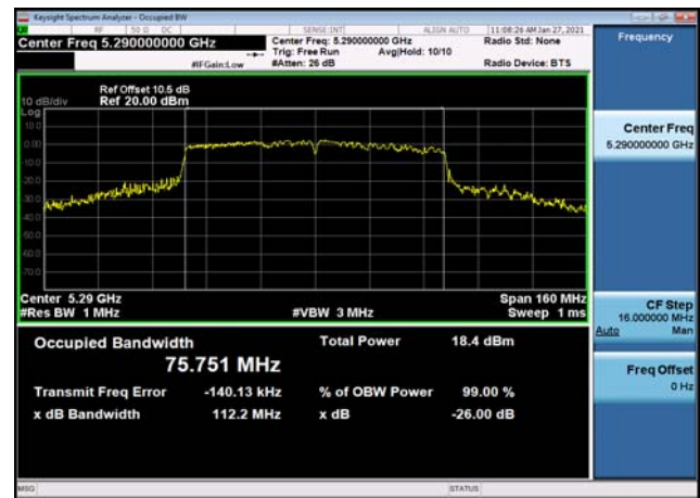
U-NII-3 99% Bandwidth-802.11n(20MHz) ,5785MHz,Ant1
