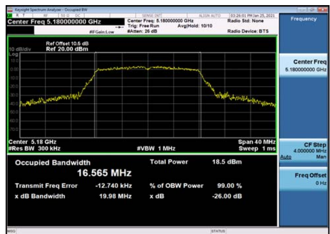
U-NII-1 99% Bandwidth-802.11a(20MHz) ,5180MHz,Ant1
