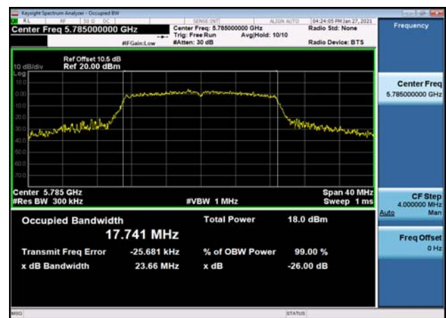
U-NII-3 99% Bandwidth-802.11n(20MHz) ,5785MHz,Ant1
