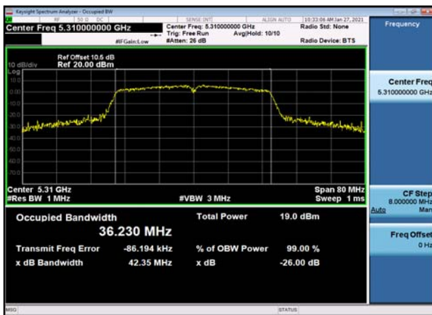
U-NII-2a 99% Bandwidth-802.11a(20MHz) ,5300MHz,Ant1
