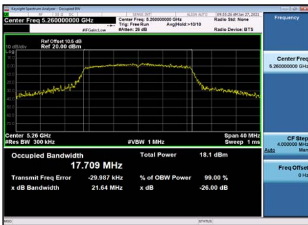
U-NII-2a 99% Bandwidth-802.11ac(20MHz) ,5260MHz,Ant1
