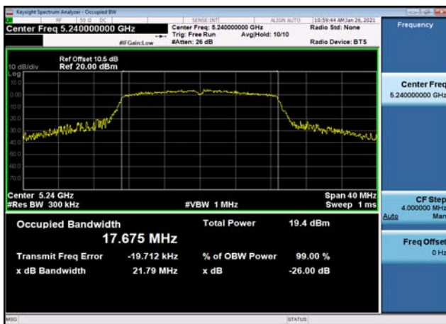
U-NII-1 99% Bandwidth-802.11n(40MHz) ,5230MHz,Ant1
