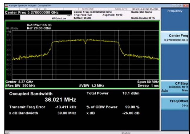
U-NII-2a 26dB Bandwidth-802.11a(20MHz )5260MHz,Ant1
