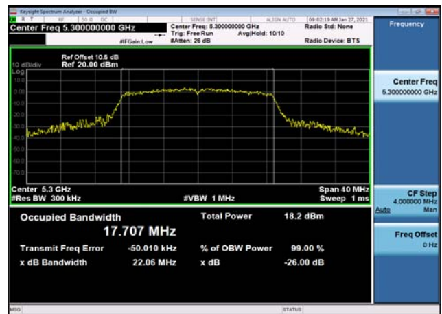
U-NII-2a 99% Bandwidth-802.11n(40MHz) ,5270MHz,Ant1
