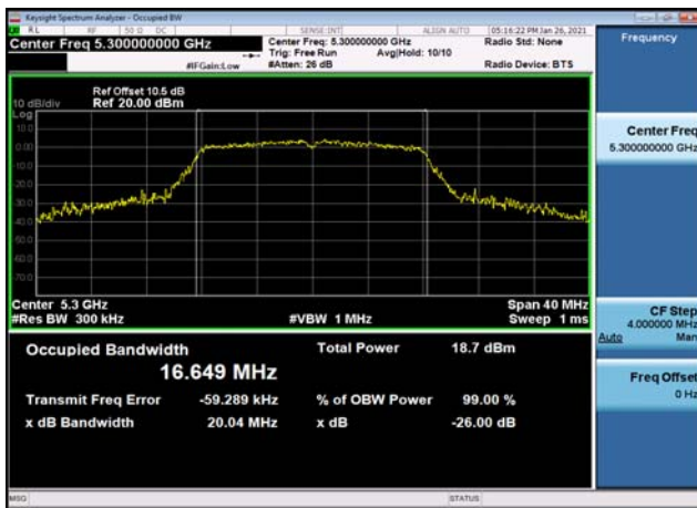
U-NII-2a 99% Bandwidth-802.11ac(20MHz) ,5260MHz,Ant1
