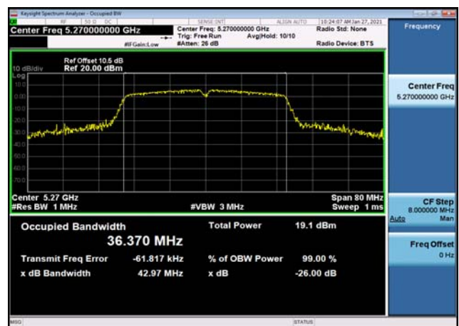
U-NII-2a 99% Bandwidth-802.11n(40MHz) ,5270MHz,Ant1
