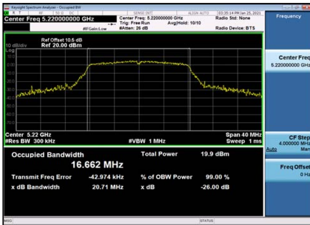
U-NII-1 99% Bandwidth-802.11ac(20MHz) ,5180MHz,Ant1
