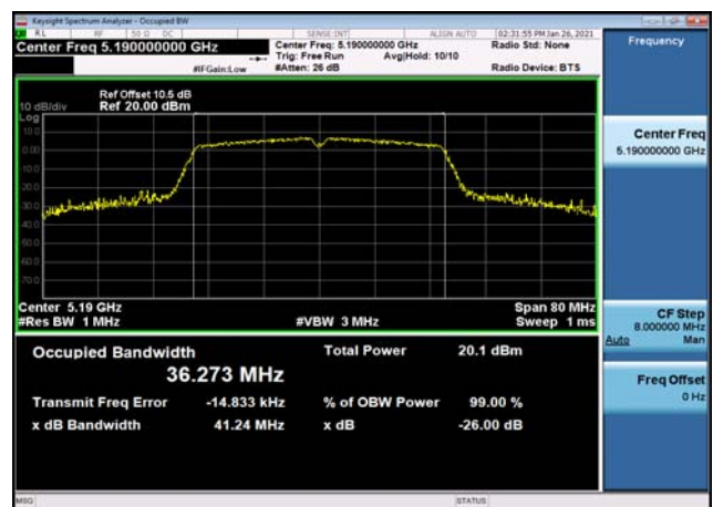
U-NII-1 99% Bandwidth-802.11ac(40MHz) ,5190MHz,Ant1
