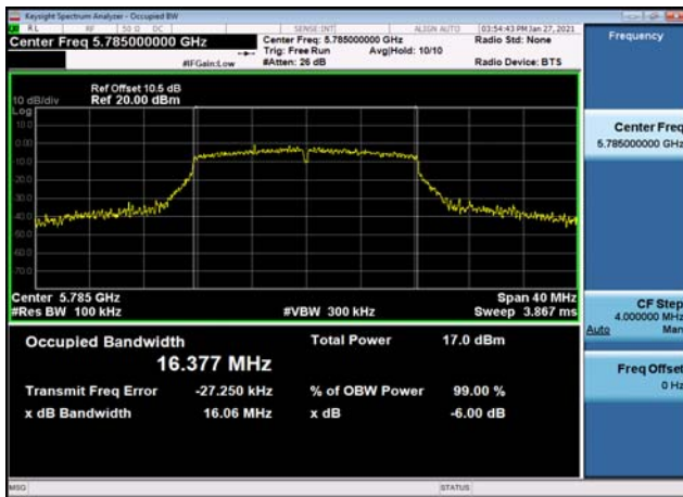
U-NII-3 6dB Bandwidth-802.11ac(20MHz) ,5745MHz,Ant1
