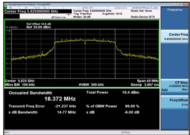
U-NII-3 6dB Bandwidth-802.11ac(20MHz) ,5785MHz,Ant1
