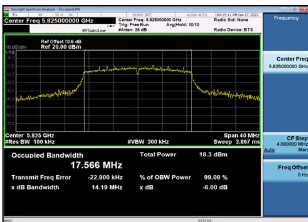
U-NII-3 6dB Bandwidth-802.11n(40MHz) ,5795MHz,Ant1
