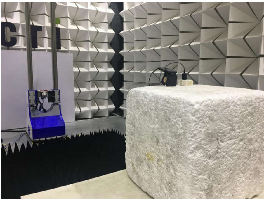
Radiated spurious emission Test Setup-2(1GHz~18GHz)
