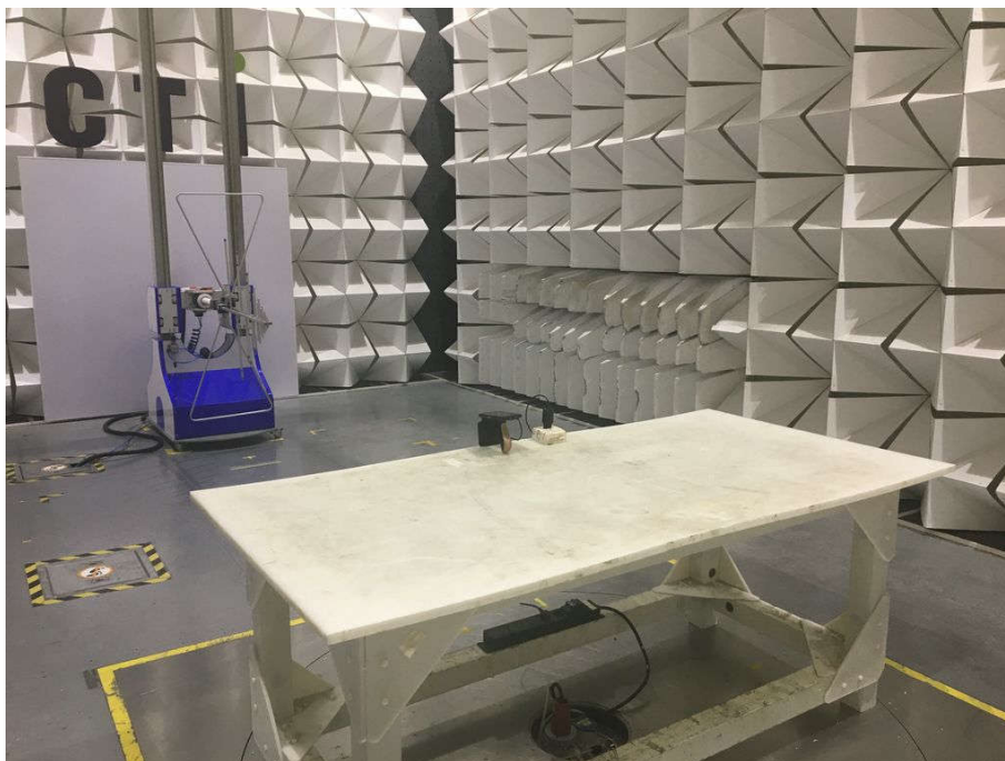
Radiated spurious emission Test Setup-1(30MHz~1GHz)
