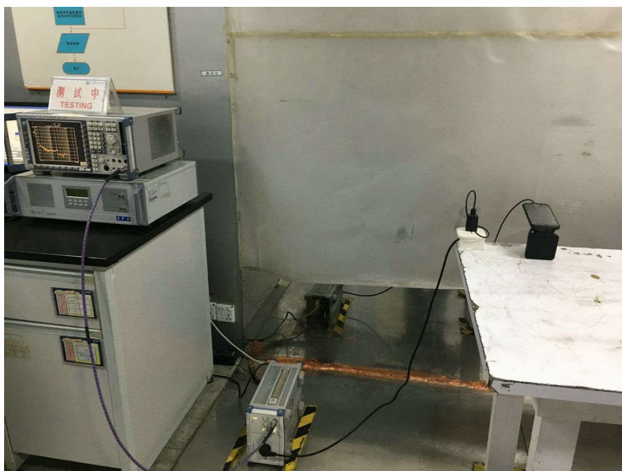
Conducted Emissions Test Setup
