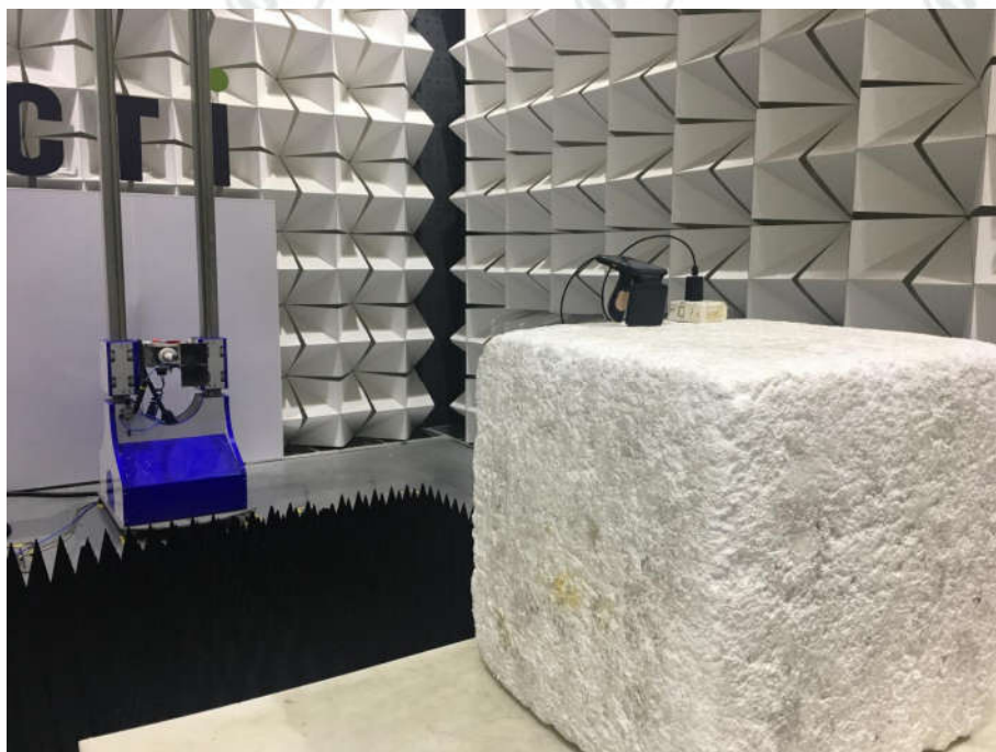
Radiated spurious emission Test Setup-2(1GHz~18GHz)
