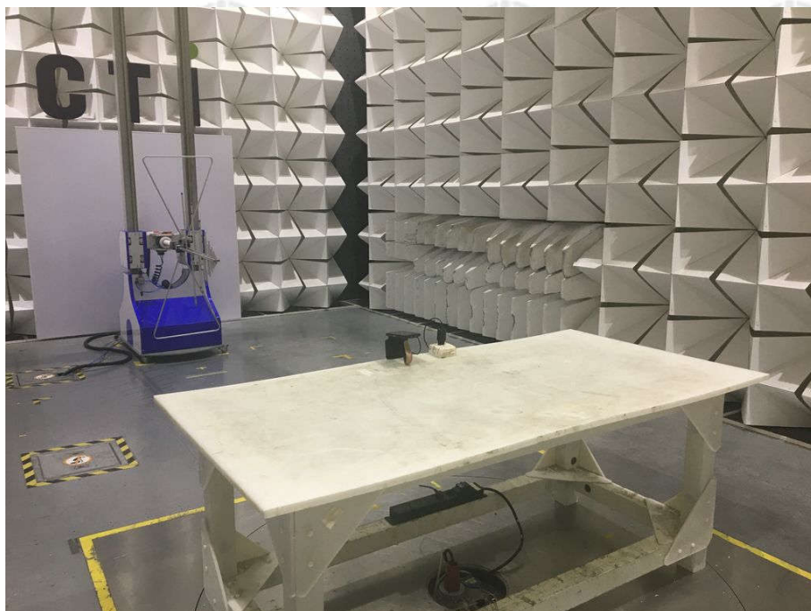
Radiated spurious emission Test Setup-1(30MHz~1GHz)
