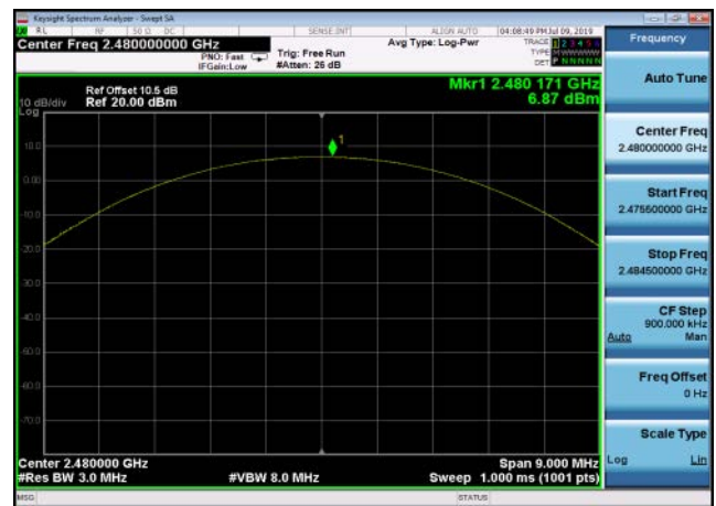
Output Power: DQPSK,2480MHz,2DH5
