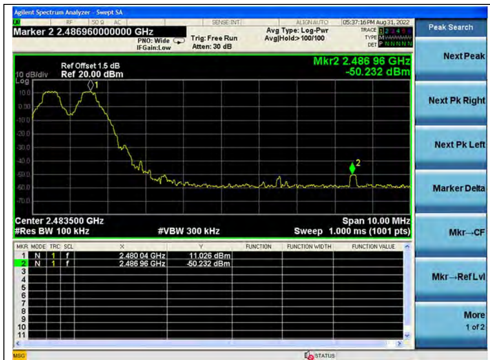
(Band edge with hopping on, Channel 78, GFSK)
