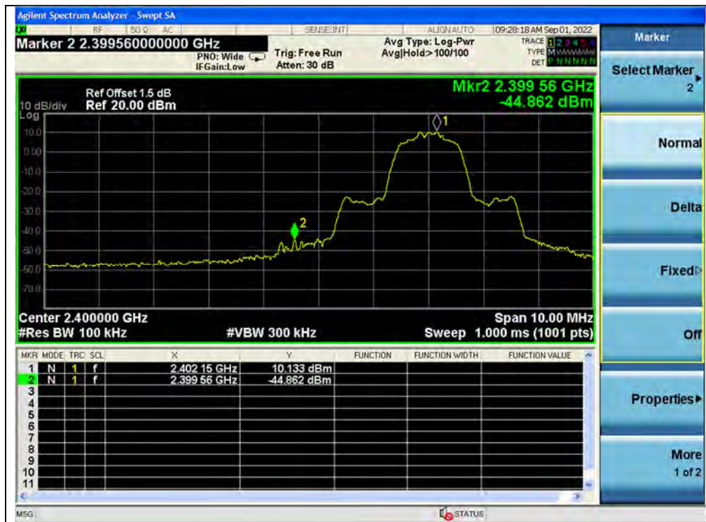
(Band edge, Channel 0, \pi/4 -DQPSK)
