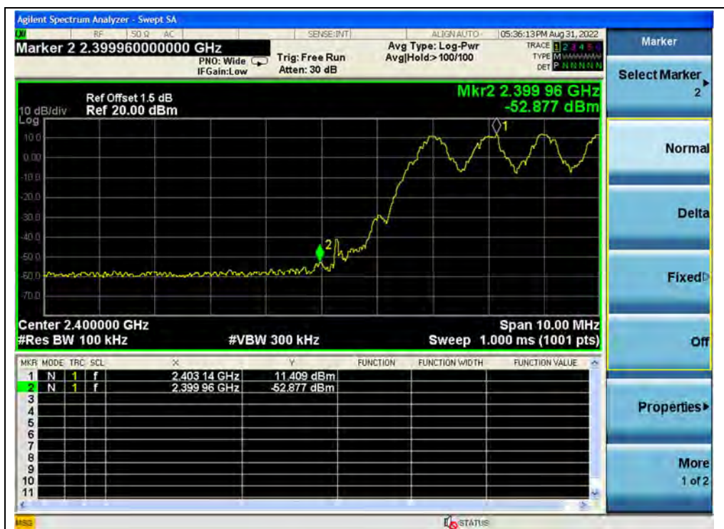
(Band edge with hopping on, Channel 0, GFSK)
