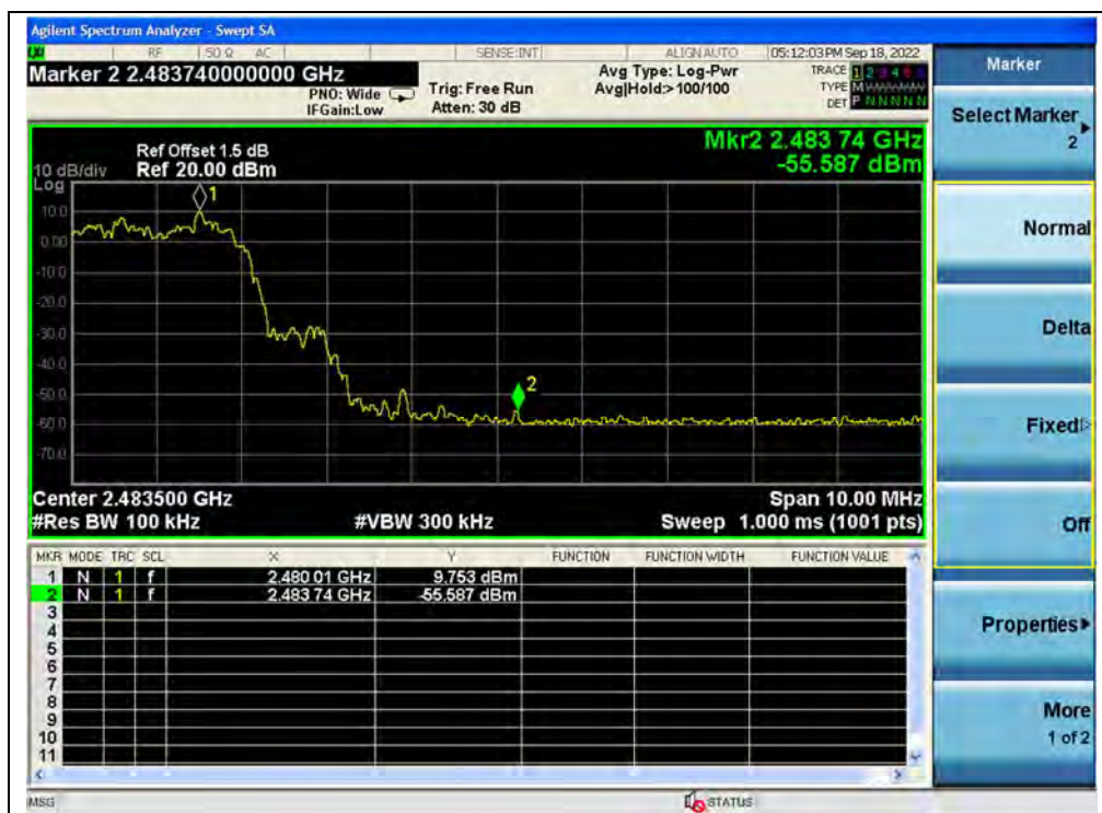
(Band edge with hopping on, Channel 78, 8-DPSK)
