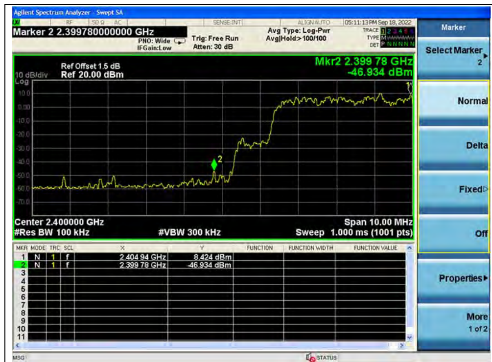
(Band edge with hopping on, Channel 0, 8-DPSK)
