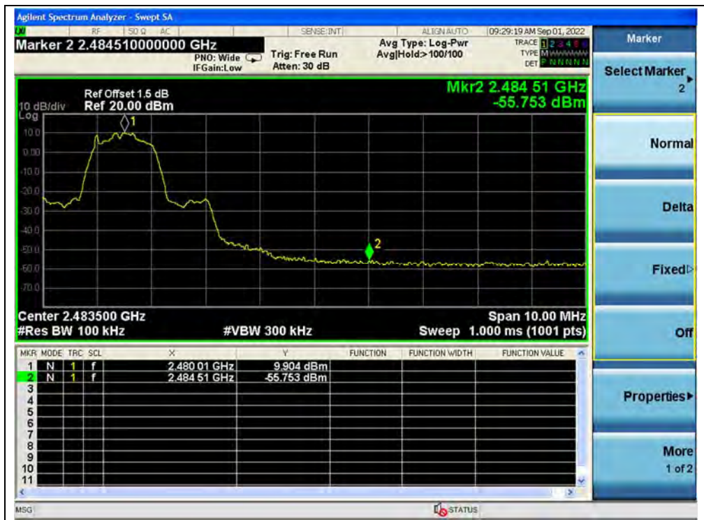
(Band edge, Channel 78, \pi/4 -DQPSK)
