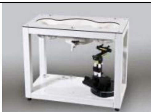
Fig. 6.8 Photo of SAM Phantom
