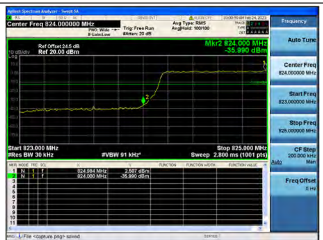
Band5 / 3MHz / Low CH / QPSK / FULL RB
