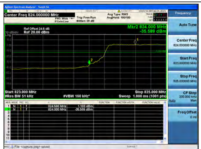
Band5 / 5MHz / Low CH / QPSK / FULL RB
