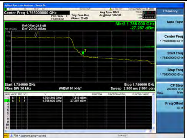
Band4 / 1.4MHz / High CH / QPSK / FULL RB
