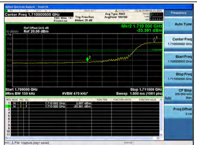
Band4 / 15MHz / Low CH / QPSK / FULL RB
