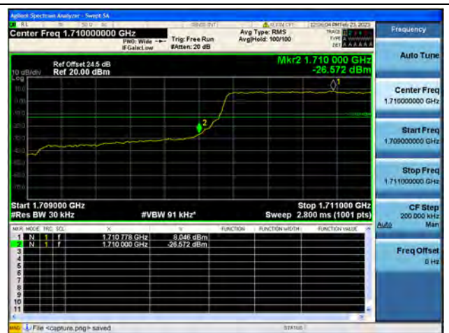
Band4 / 1.4MHz / Low CH / QPSK / FULL RB
