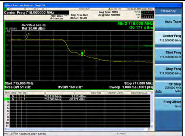
Band12 / 5MHz / High CH / QPSK / FULL RB
