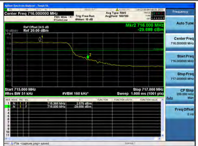
Band17 / 5MHz / High CH / QPSK / FULL RB
