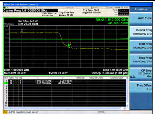
Band2 / 3MHz / High CH / QPSK / FULL RB
