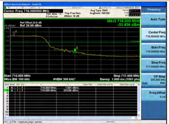
Band12 / 10MHz / High CH / QPSK / FULL RB
