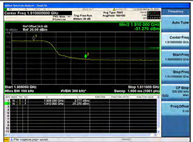
Band2 / 10MHz / High CH / QPSK / FULL RB
