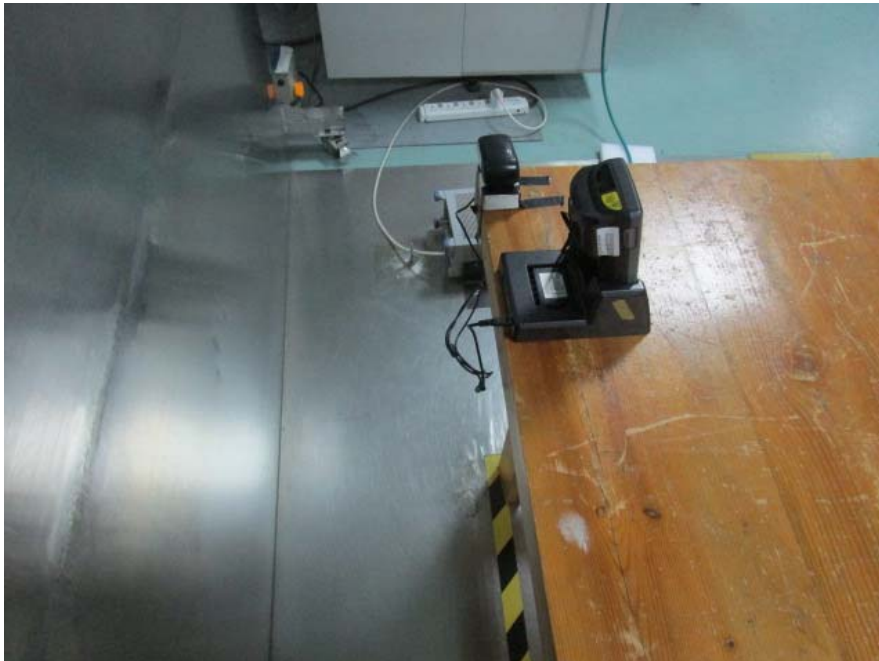
Conducted Emissions –Side View
