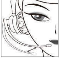
To avoid low or distorted sound, and to provide clear and crisp telephone calls, the microphone should be positioned within 30-40mm of your mouth. The microphone boom arm will move in a variety of directions to ensure the best fit.
