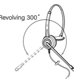
To change side, rotating the microphone boom over the headband to accommodate the left or right ear.
