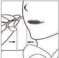
Your new headset is supplied with a clothing clip to allow comfortable fitting of your headset without the cable getting caught or inadvertently pulled. The clothing clip should be fastened at a comfortable level, ensuring that there is sufficient slack on the cable allowing free movement of your head without disturbing the headset position.
