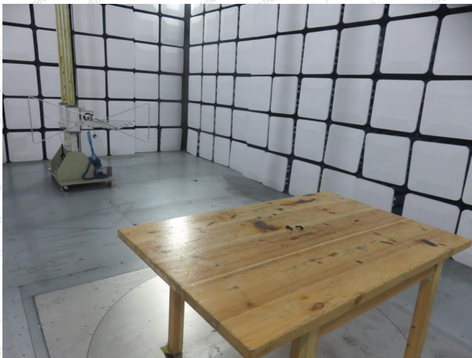
Photo of Radiation Emission Test
