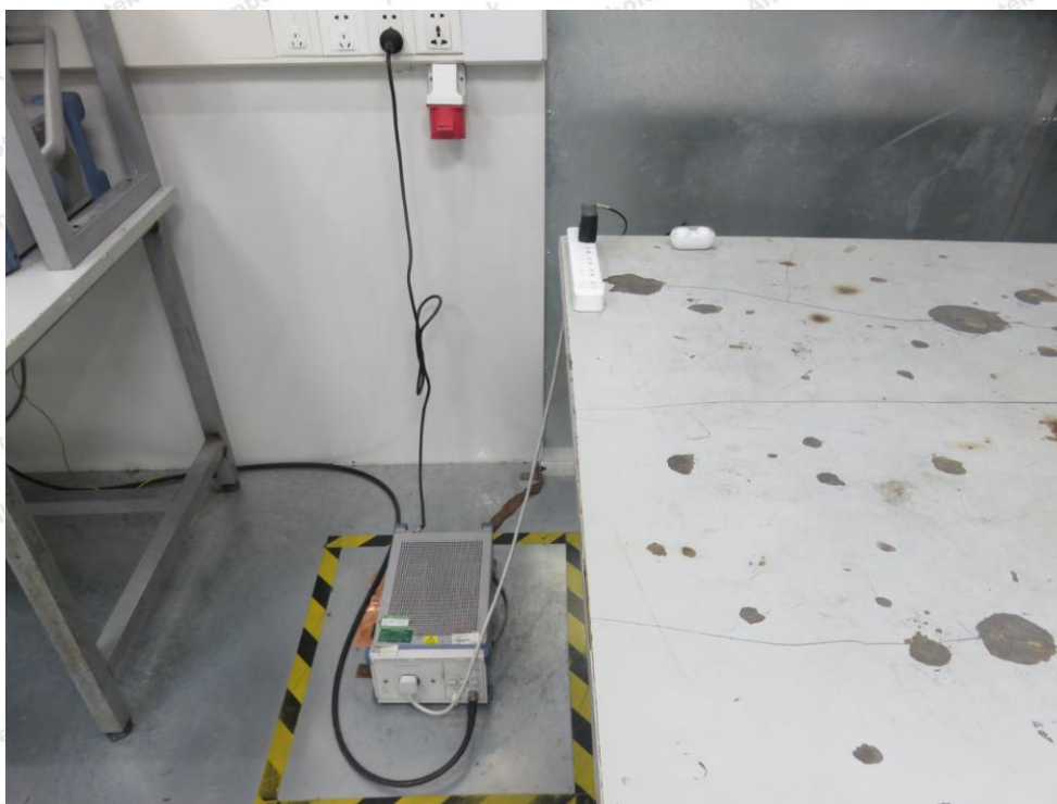
Photo of Conducted Emission Measurement
