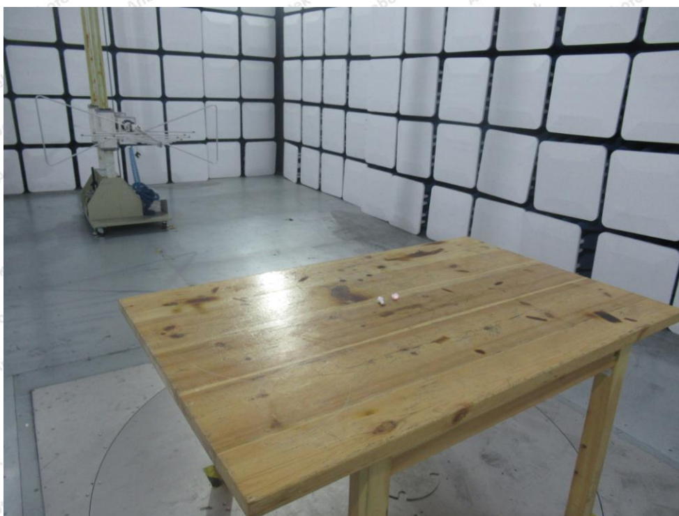
Photo of Radiation Emission Test
