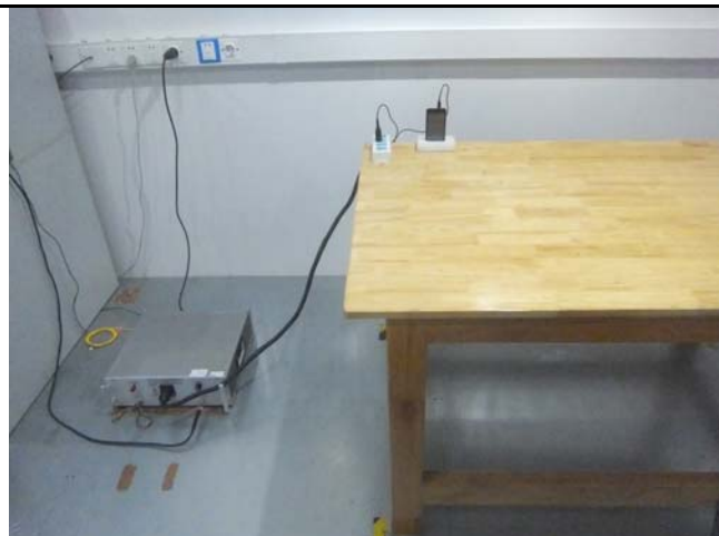
Conducted Emissions Test Setup Front View
