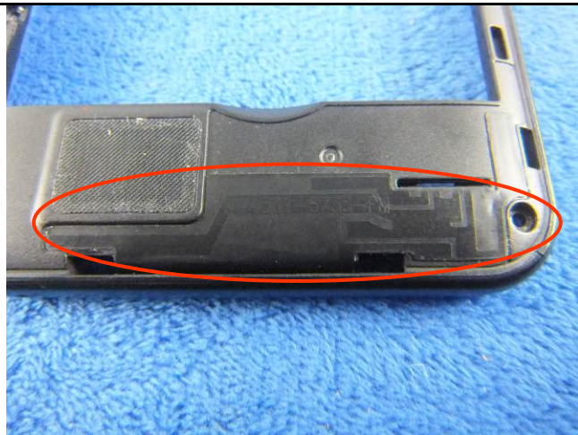
GSM/PCS/UMTS-FDD Antenna View
