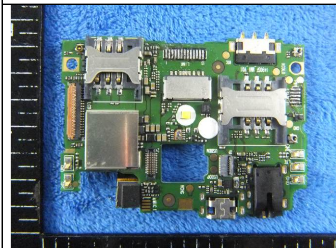
Mainboard with Shielding - Front View
