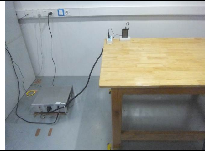
Conducted Emissions Test Setup Front View
