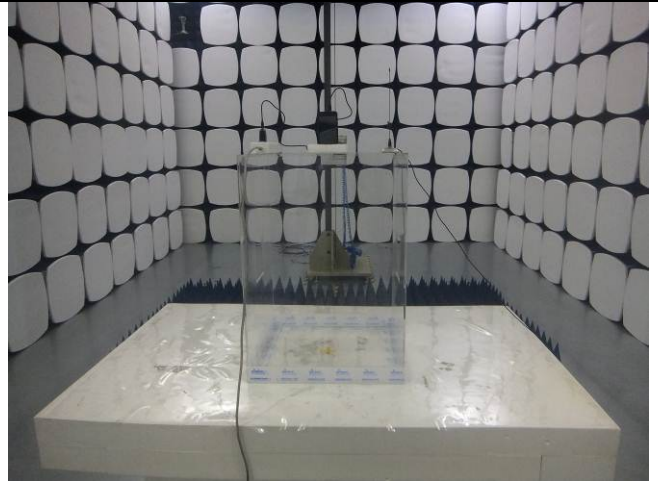
Radiated Spurious Emissions Test Setup Above 1GHz
