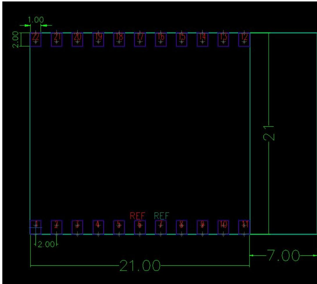
The module is a "solderable module and therefore the pad dimensions must be followed exactly.
