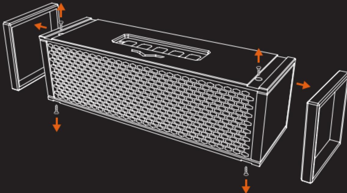
3. Remove the pre-installed housing
