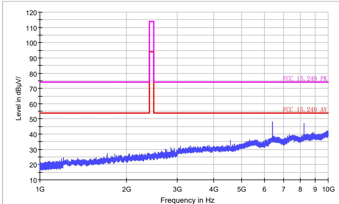
Transmitting at 916MHz, above 1GHz, Horizontal
