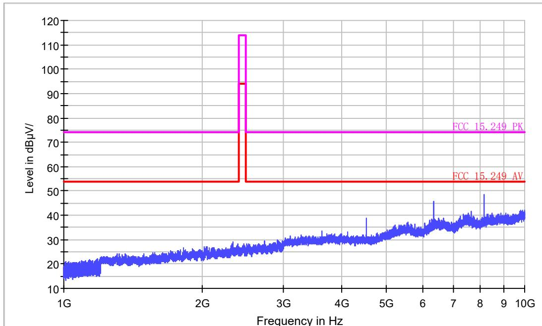
Transmitting at 908.4MHz, above 1GHz, Horizontal
