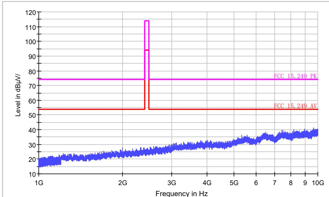
Transmitting at 908.4MHz, above 1GHz, Horizontal
