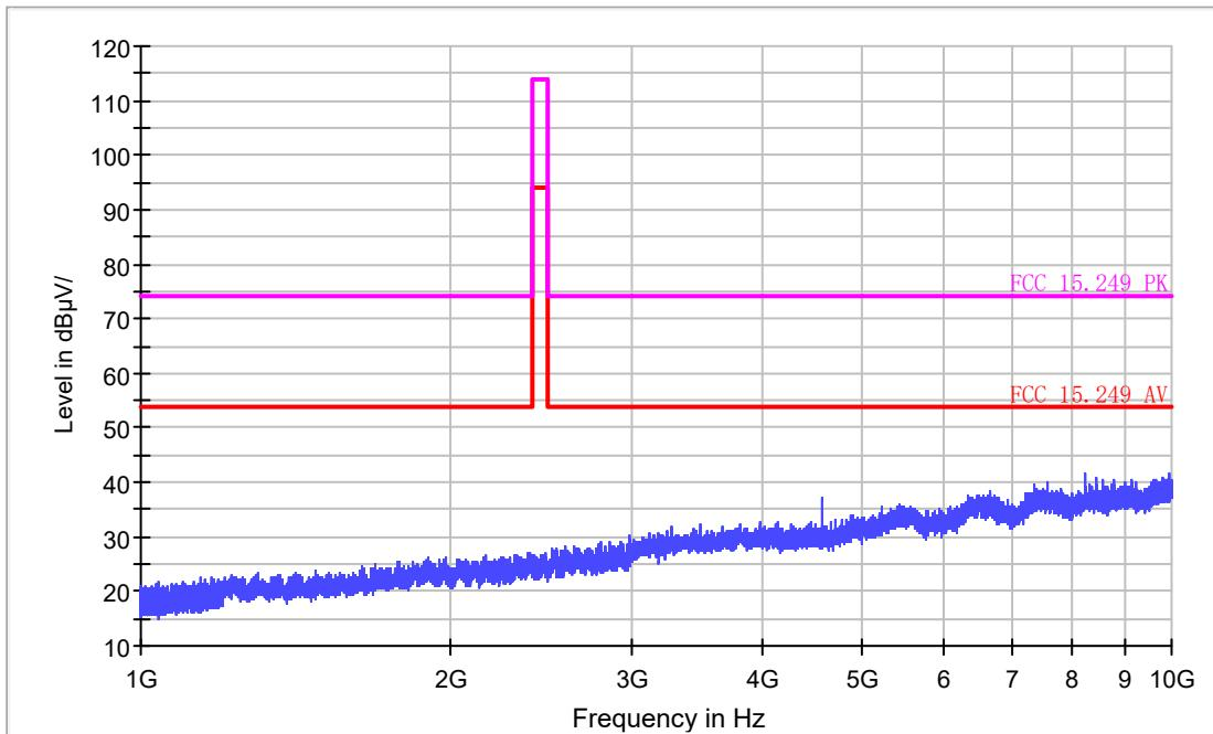
Transmitting at 916MHz, above 1GHz, Horizontal
