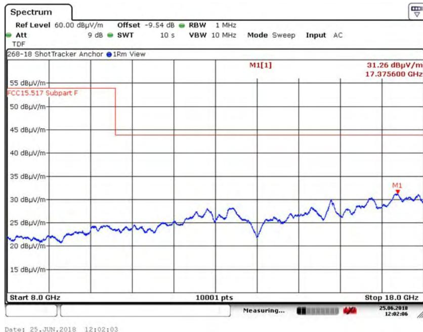
6.5.14. 8 to 18 GHz Vertical at 1 Meter, -9.54 dB offset in analyzer CH3, 16M
