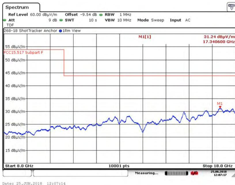
6.5.16. 8 to 18 GHz Vertical at 1 Meter, -9.54 dB offset in analyzer CH3, 64M
