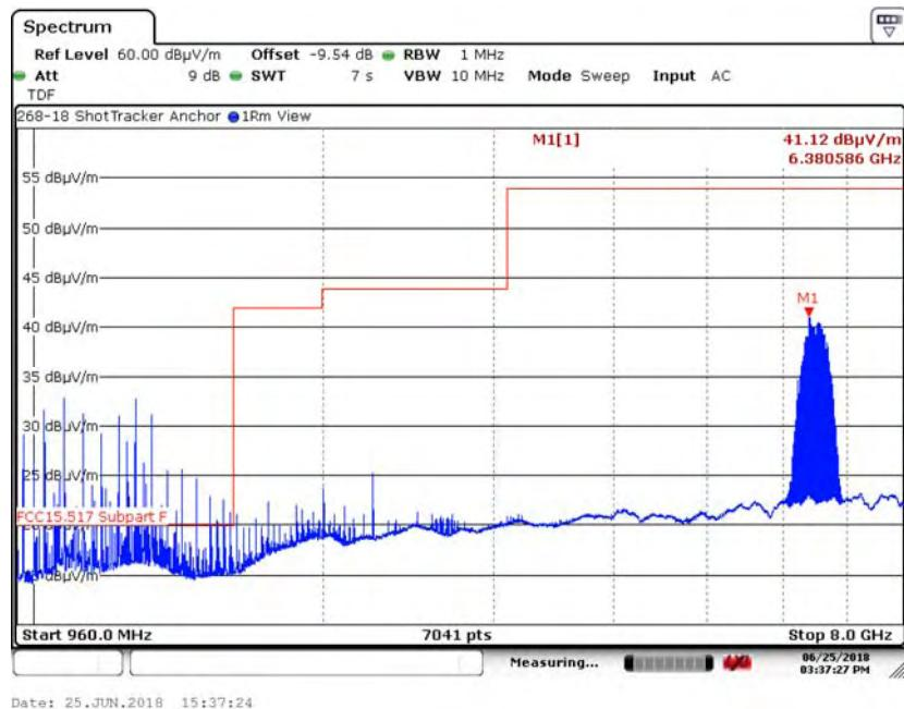
6.5.6. 960 MHz to 8 GHz Vertical at 1 Meter, -9.54 dB offset in analyzer CH5,16M
