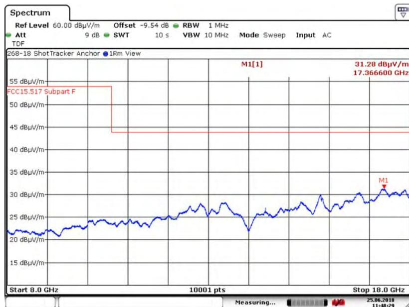
6.5.24. 8 to 18 GHz Vertical at 1 Meter, -9.54 dB offset in analyzer CH7, 64M
