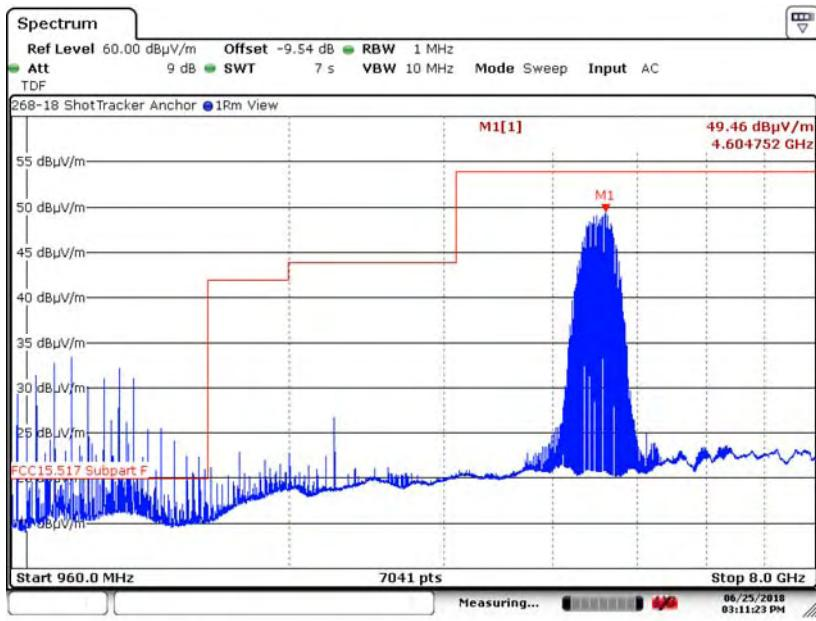
6.5.4. 960 MHz to 8 GHz Vertical at 1 Meter, -9.54 dB offset in analyzer CH3,64M
