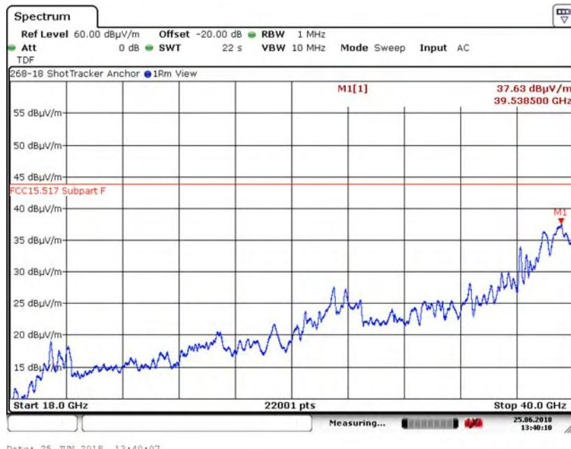
6.5.28. 18 to 40 GHz Vertical at 0.5 Meter, -15.56 dB offset in analyzer CH3, 64M
