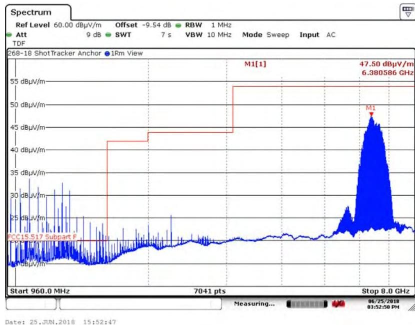
6.5.12. 960 MHz to 8 GHz Vertical at 1 Meter, -9.54 dB offset in analyzer CH5,64M
