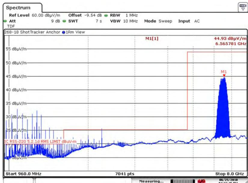
6.5.40. 960 MHz to 8 GHz Vertical at 1 Meter, -9.54 dB offset in analyzer CH5,64M
