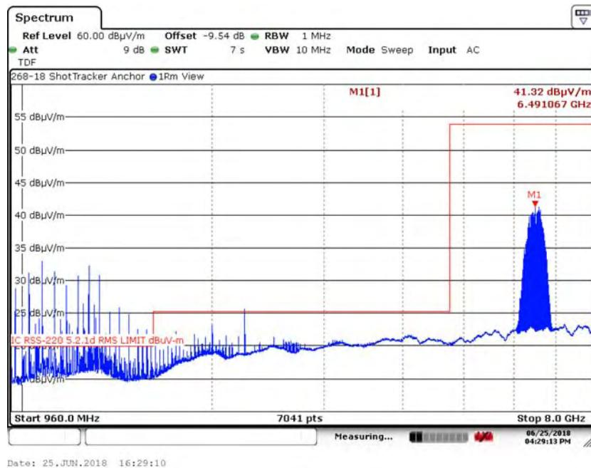
6.5.38. 960 MHz to 8 GHz Vertical at 1 Meter, -9.54 dB offset in analyzer CH5,16M
