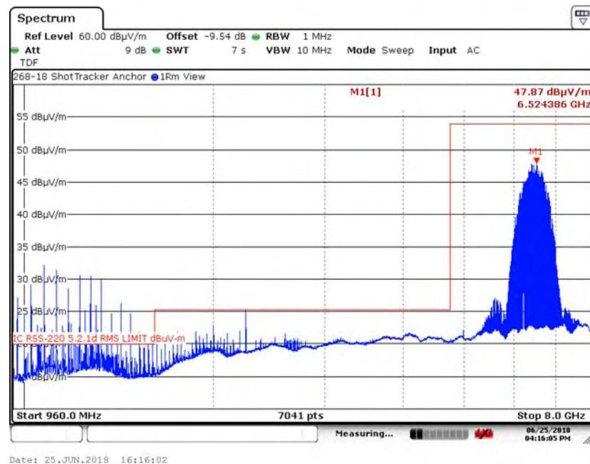
6.5.44. 960 MHz to 8 GHz Vertical at 1 Meter, -9.54 dB offset in analyzer CH7,64M
