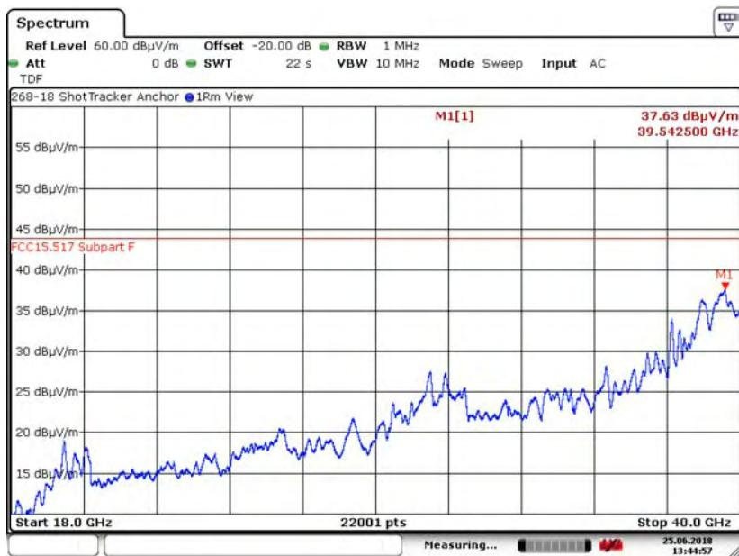
6.5.26. 18 to 40 GHz Vertical at 0.5 Meter, -15.56 dB offset in analyzer CH3, 16M
