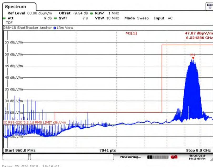
6.5.42. 960 MHz to 8 GHz Vertical at 1 Meter, -9.54 dB offset in analyzer CH7,16M
