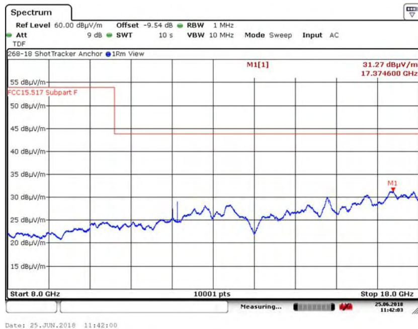
6.5.22. 8 to 18 GHz Vertical at 1 Meter, -9.54 dB offset in analyzer CH7, 16M
