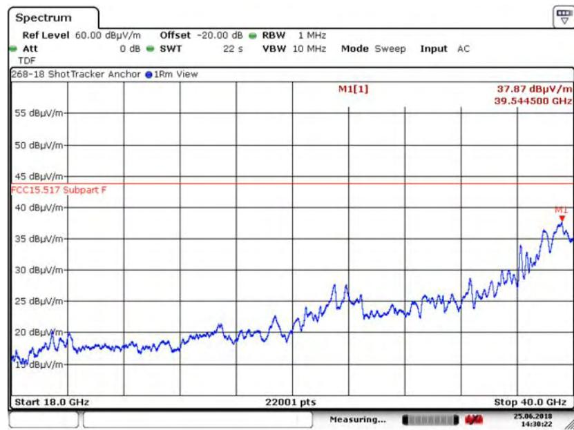
6.5.34. 18 to 40 GHz Vertical at 0.5 Meter, -15.56 dB offset in analyzer CH7, 16M
