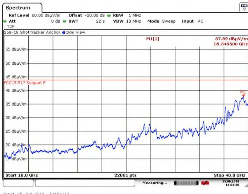
6.5.32. 18 to 40 GHz Vertical at 0.5 Meter, -15.56 dB offset in analyzer CH5, 64M
