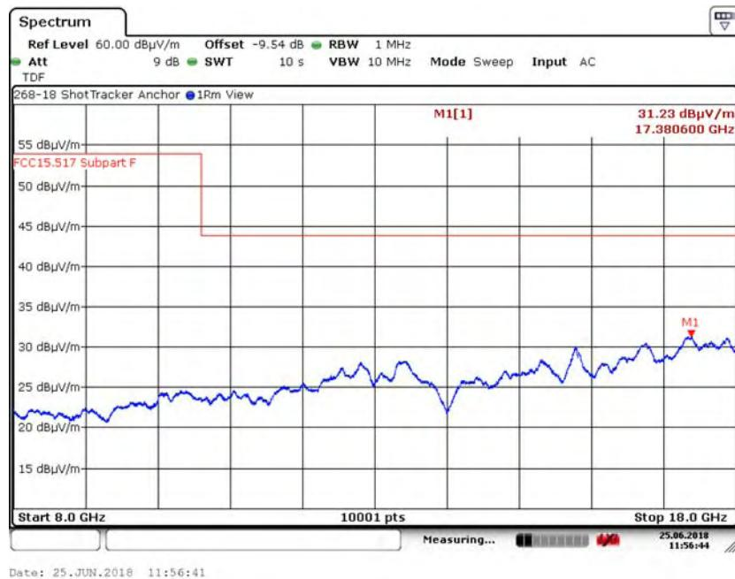
6.5.20. 8 to 18 GHz Vertical at 1 Meter, -9.54 dB offset in analyzer CH5, 64M
