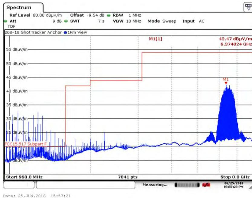
6.5.10. 960 MHz to 8 GHz Vertical at 1 Meter, -9.54 dB offset in analyzer CH7,16M
