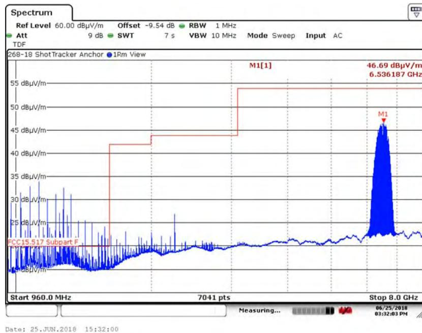
6.5.8. 960 MHz to 8 GHz Vertical at 1 Meter, -9.54 dB offset in analyzer CH5,64M
