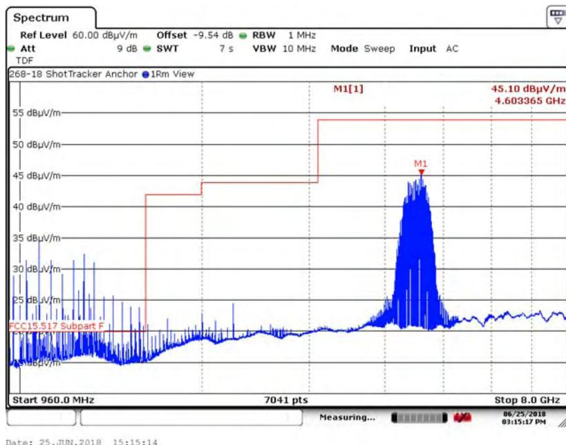
6.5.2. 960 MHz to 8 GHz Vertical at 1 Meter, -9.54 dB offset in analyzer CH3,16M
