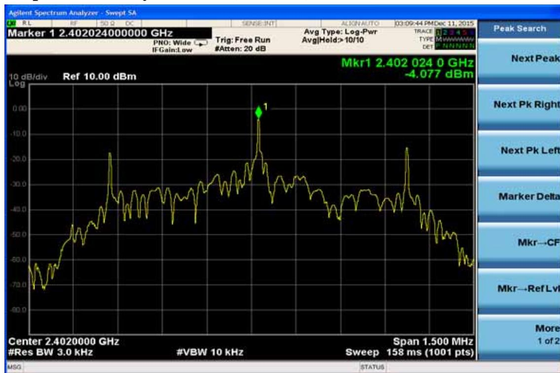
**Power Spectral Density Test Plot (CH-Mid)**
