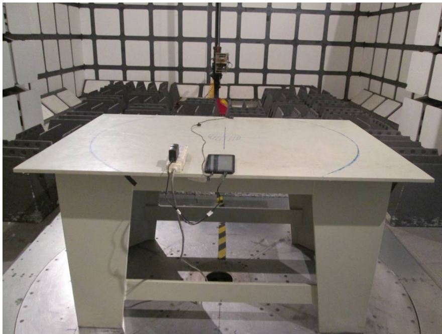
Radiated Emissions – Rear View (1-25 GHz)
