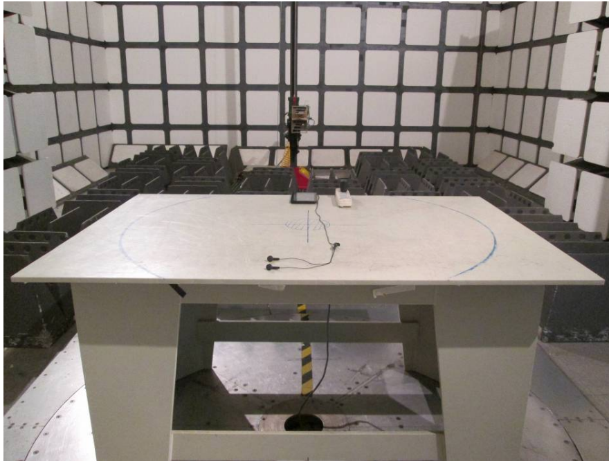
Radiated Emissions – Front View (1-25 GHz)
