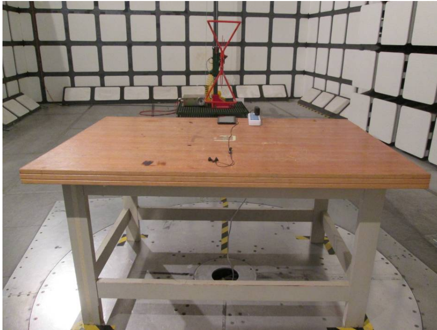
Radiated Emissions – Front View (30-1000 MHz)
