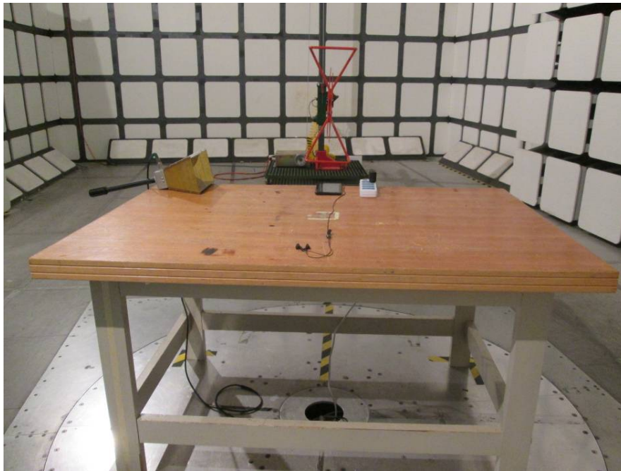
Radiated Emissions - Front View (Below 1GHz)
