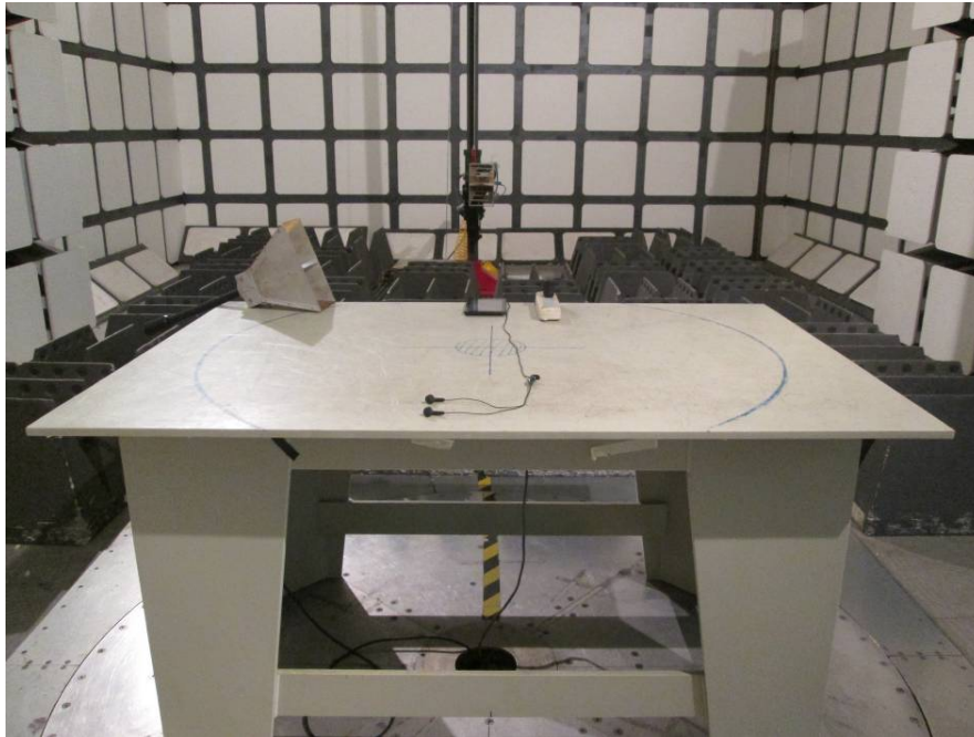
Radiated Emissions - Front View (Above 1GHz)
