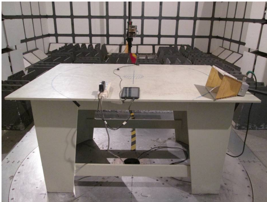
Radiated Emissions - Rear View (Above 1GHz)
