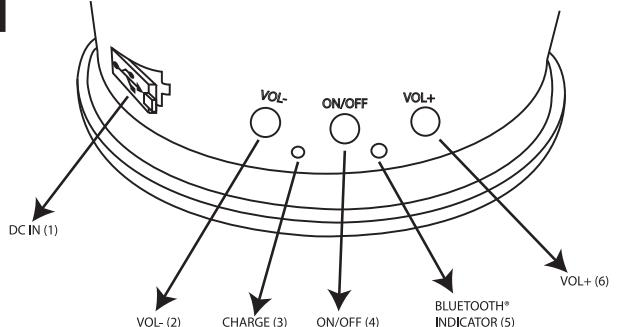
**NOTE:** The ON/OFF button (4) controls both the Bluetooth® connection and the flickering candle light.
