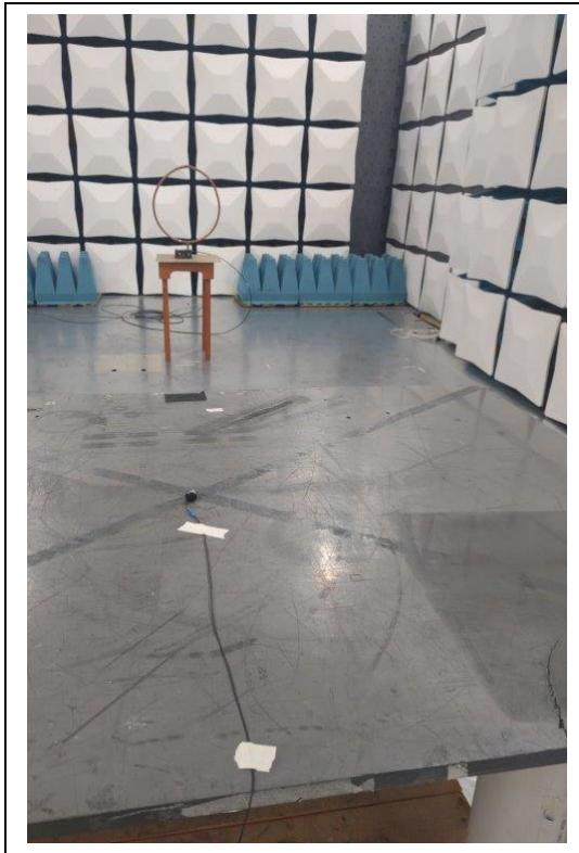
**Radiated Emissions: 30 MHz to 1000 MHz**
